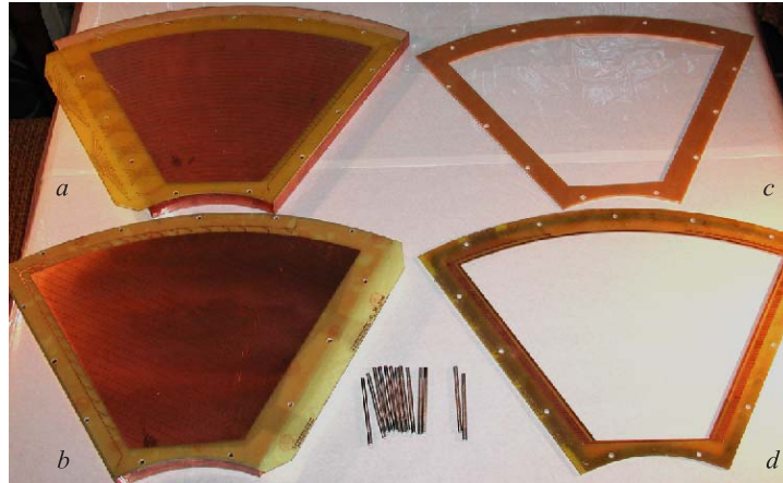
Fig. 5. Parts of MWPC made on SKLUST of sizes 460 \times 350 \text{ mm}^2 : cathode planes with strips ( a, b ), the spacer frame ( c ), the anode frame ( d )
