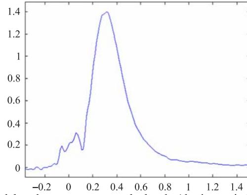
Fig. 4. Additional delayed neutron source calculated. Abscissa axis is time in ms, axis of ordinates is  $S(t)$
