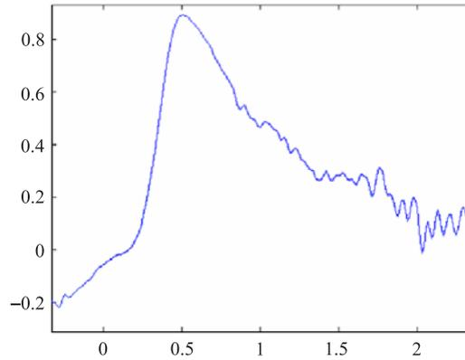
Fig. 3. Relative difference in  $N(t)$  :  $(N_{\text{exp}}(t) - N_{\text{calc}}(t)) / N_{\text{exp}}(t) = S_{\text{th}} / (S_{\text{th}} + S_{\text{delayed}})$ . Abscissa axis is time in msec, axis of ordinates is relative difference in  $N(t)$
