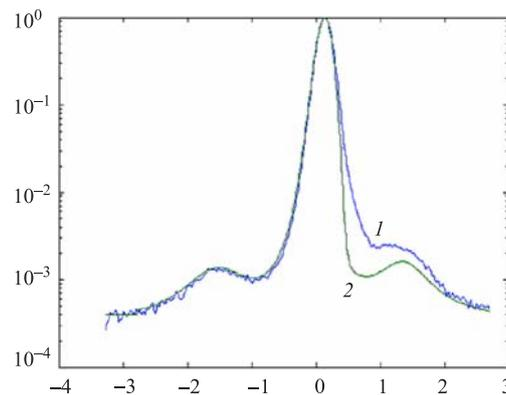
Fig. 1. Measured (1) and calculated (2) reactor pulse of the IBR-2 reactor with PO-3 moving reflector. Abscissa axis is time in ms, axis of ordinates is equivalent to  $N(t)$  used in the text
