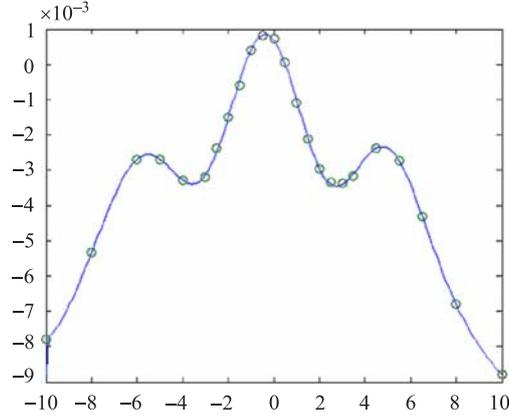
Fig. 2. Reactivity in parts of  $K_{\text{eff}}$  versus position of the moving reflector (measurement at subcritical state of the reactor with «reversed multiplication» method and shifted up to critical state). Abscissa axis is displacement of the main moving reflector OPO from the position of maximum reactivity
