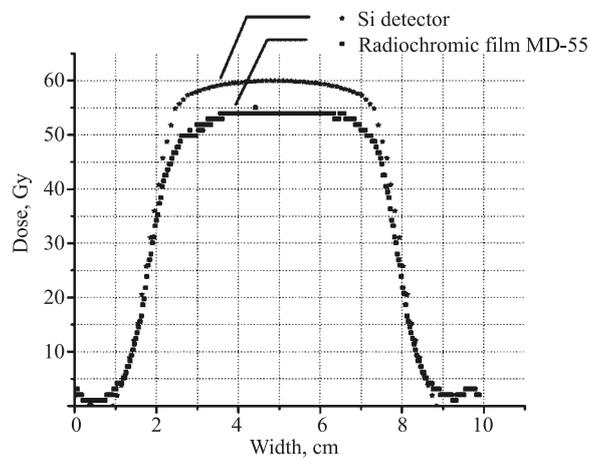
Fig. 3. Comparison of horizontal profiles measured in the Bragg peak region
