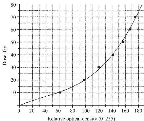
Fig. 1. Calibration curve of type MD-55 radiochromic film obtained with a Vidar-16 scanner
