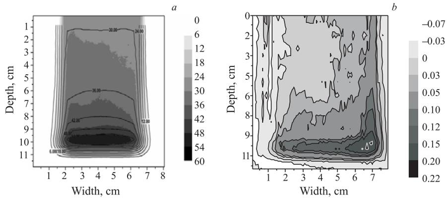
Fig. 2. Isodoses obtained from the radiochromic film (in gray-scale representation) and with the Si-semiconductor detector (in lines) for an unmodulated beam (a) and differences between the RCF and the Si detector on the plane (b)
