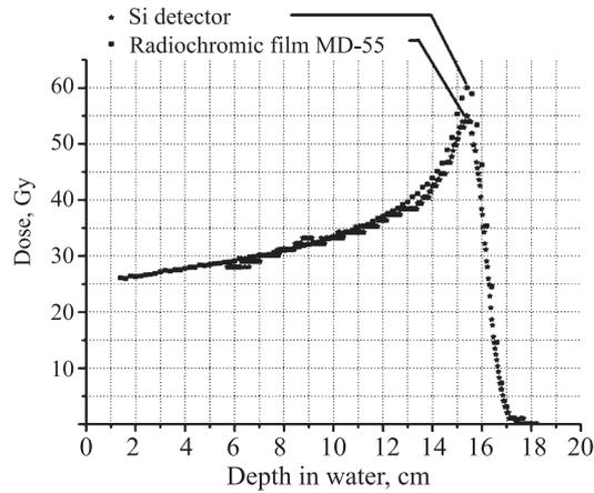
Fig. 4. Comparison of the Bragg curves along the central axis
