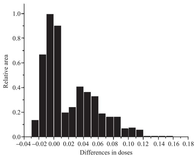
Fig. 7. Histogram of differences between doses obtained with the RCF and the Si detector for a modulated beam
