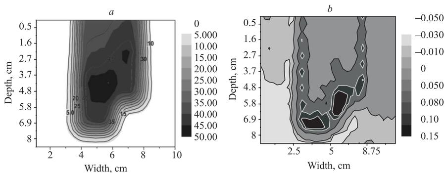
Fig. 6. Isodoses obtained from the radiochromic film (gray-scale representation) and with the Si-semiconductor detector (lines) for a beam modulated with a ridge filter and a bolus (a) and differences between the measurements with the RCF and the Si detector on the plane (b)
