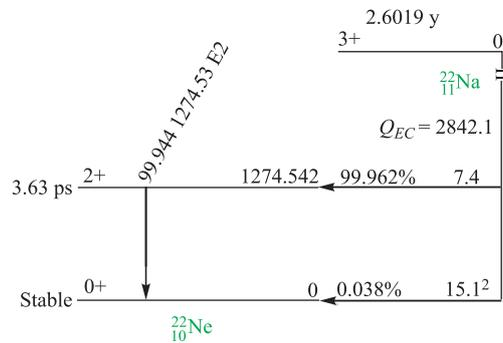
Fig. 1. The decay scheme of  $^{22}\text{Na}$  [16]
