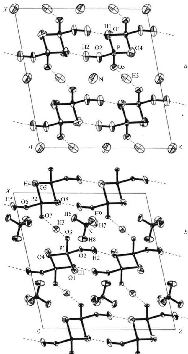
Fig. 1. The projection on  $X0Z$  plane of crystal structure of  $\text{NH}_4\text{H}_5(\text{PO}_4)_2$ : (a) — high temperature phase, (b) — low temperature phase. The thermal ellipsoids are given with 50% probability, only hydrogen bonds of the type  $\text{O}-\text{H}\dots\text{O}$  are shown by dashed lines
