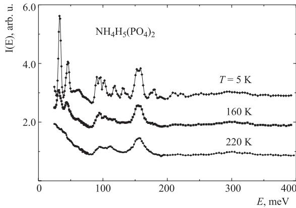
Fig. 2.  $\text{NH}_4\text{H}_5(\text{PO}_4)_2$ , obtained inelastic incoherent neutron scattering (IINS) spectra at 5 K and before and after phase transition at temperatures 160 and 220 K, respectively
