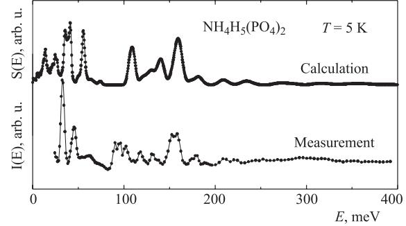
Fig. 3. The comparison of the IINS( $E$ ) spectrum of  $\text{NH}_4\text{H}_5(\text{PO}_4)_2$ , measured at 5 K, and  $S(E)$  spectrum, calculated for low temperature phase
