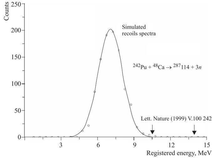
Fig. 6. Recoil spectrum simulation for recoil signal amplitudes reported in [21]. Measured (two events) deviate from calculations by  $\sim 40$  and  $90\%$ , respectively
