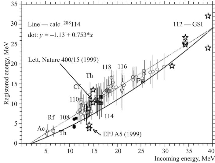
Fig. 1. Dependence of the registered recoil energy signal against incoming one. Calculation of [17] is shown by line. Dotted line is plotted to guide the eye — direct empirical calibration [18] measured for different heavy recoils at the DGFRS. Data of the SHIP and VASSILISSA are shown by stars
