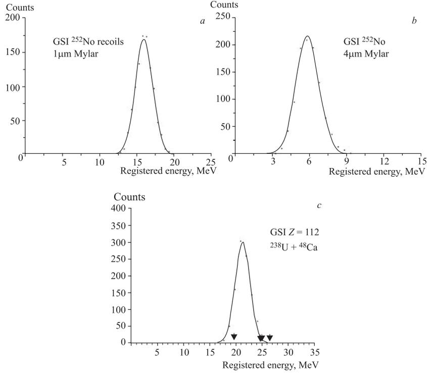
Fig. 2. Simulation of the registered energy spectra of EVRs of  $^{252}\text{No}$  for experiment reported in [8]: *a*) with 1  $\mu\text{m}$  Mylar; *b*) 4  $\mu\text{m}$  Mylar degraders; *c*) simulation for  $Z = 112$  recoils from  $^{238}\text{U} + ^{48}\text{Ca} \rightarrow 112 + 3n$  reaction
