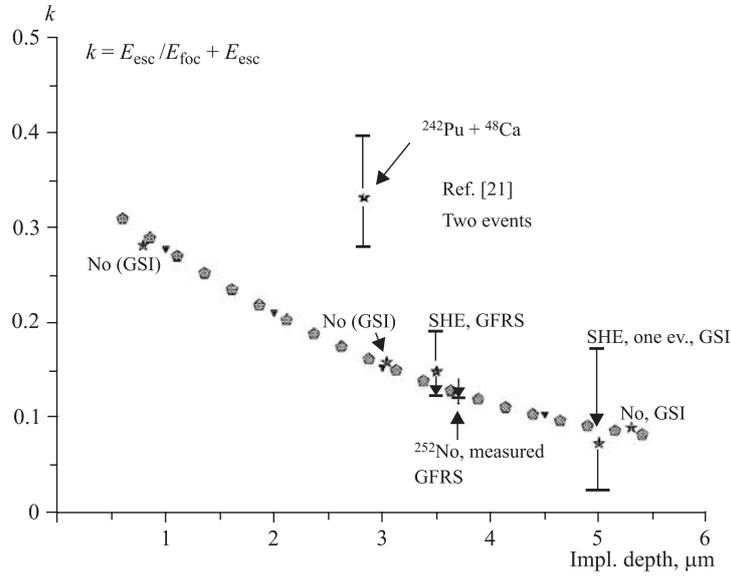
Fig. 5. The calculated dependence of  $k$  parameter against EVR implantation depth. Stars denote the values measured at different facilities
