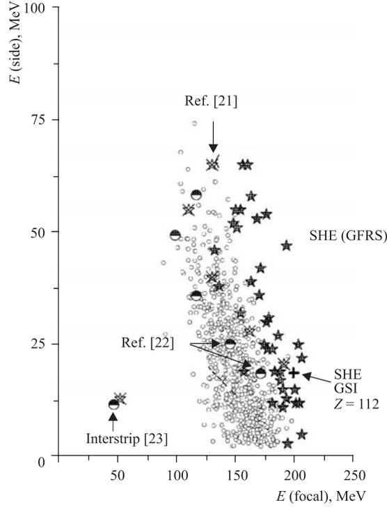
Fig. 4. Two-dimensional plot: energy registered in the main detector energy vs. that in the side detector. Open circles —  $^{252}\text{No}$ ; stars — SHE SF events measured at the DGFRS; semi-filled circles — measured at the VASSILISSA with reverse recalculation to « $\alpha$ -calibration» (star + cross — original data [21–23]); cross —  $Z = 112$  (GSI)
