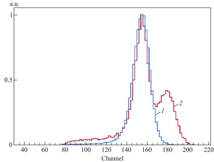
Fig. 4. Amplitude spectrum of the signals recorded by an  $\alpha$  pixel without coincidence with the signal from the gamma detector
