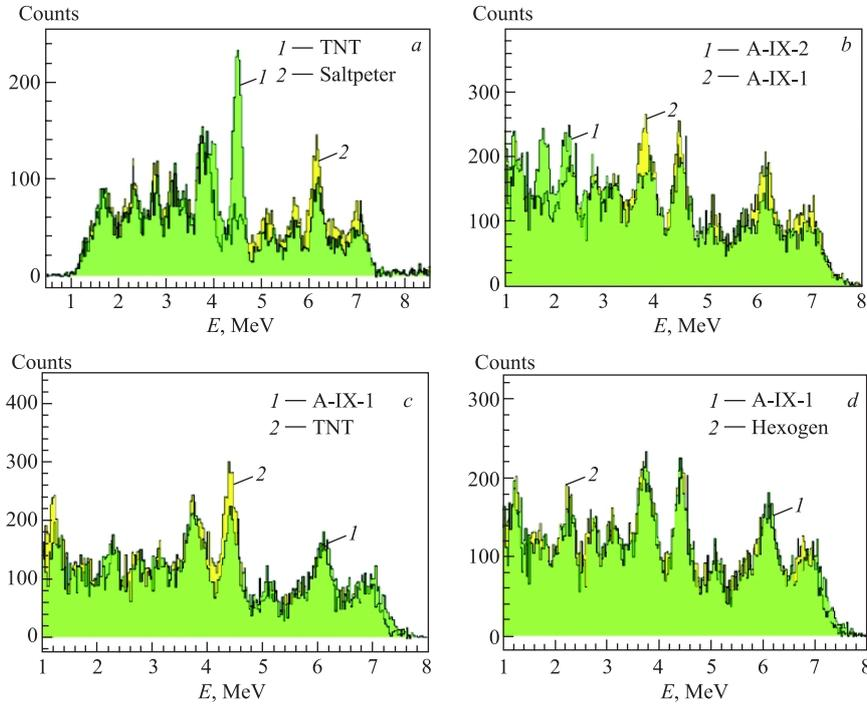
Fig. 10. The energy spectra of  $\gamma$  quanta for different explosives: *a*) TNT (1) and saltpeter (2); *b*) A-IX-2 (1) and A-IX-1 (2); *c*) TNT (2) and A-IX-1 (1); *d*) A-IX-1 (1) and hexogen (2)
