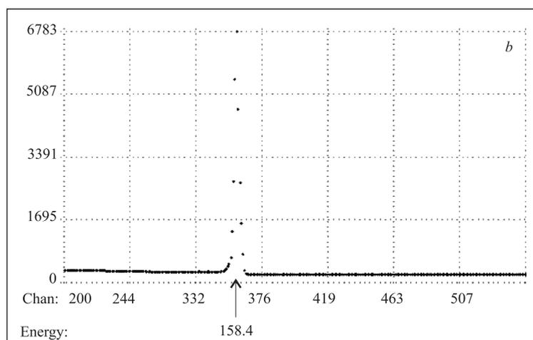
Fig. 2. a) A part of radioisotope spectrum of the irradiated natural pure Sn granule (163.5 mg); b) a part of radioisotope spectrum of the irradiated enriched  $^{118}\text{Sn}$  (98.5%) foil (30.4 mg)
