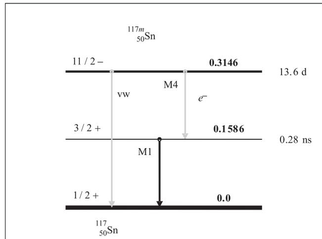
Fig. 1. The level scheme of simple energy of  ${}^{117m}\text{Sn}$
