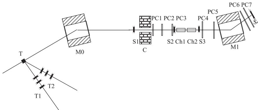
Fig. 5.  $T_i$ ,  $S_i$ , — scintillator telescopes and counters,  $Ch_i$  — Čerenkov counters,  $PC_i$  — proportional chambers,  $T$  — target,  $M_0$ ,  $M_1$  — separating and analyzing magnets
