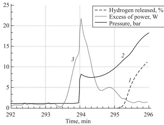
Fig. 10. Internal heat release (curve 3, W) at the first stage of heating of irradiated methane. Curve 1 — hydrogen release, %; curve 2 — pressure on the membranes, bar
