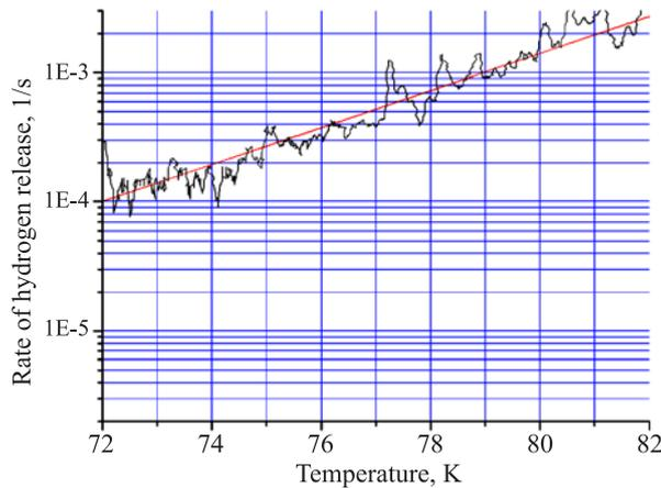
Fig. 8. Rate of hydrogen release (relative to the amount of hydrogen unreleased)
