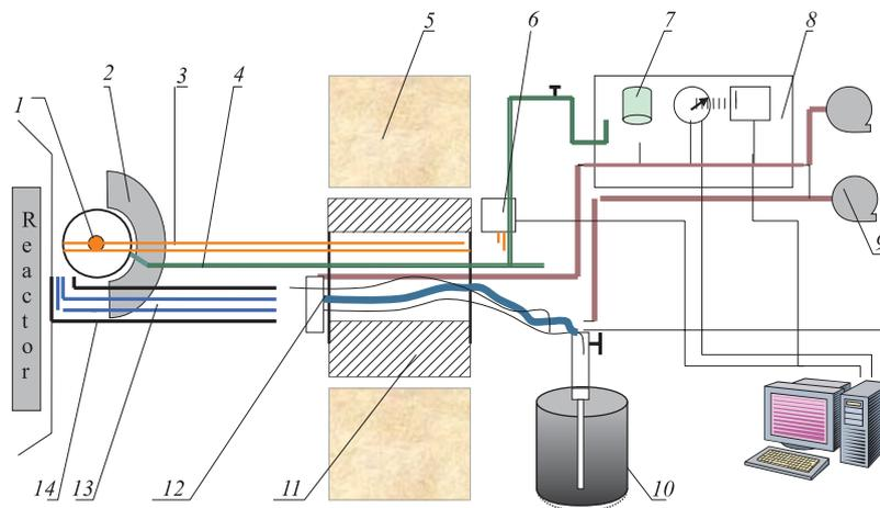
Fig. 1. The URAM-3M irradiation facility: 1 — chamber with a sample; 2 — beryllium reflector; 3 — coaxial cables of displacement gauges; 4 — methane supply pipe; 5 — biological shield of the reactor; 6 — electric adapters and amplifiers; 7 — methane and hydrogen bottles; 8 — technology console; 9 — vacuum pumps; 10 — liquid helium 200 l Dewar; 11 — movable shielding plug; 12 — flexible helium pipeline of 12 m long; 13 — straight helium pipeline; 14 — evacuated and holding tube
