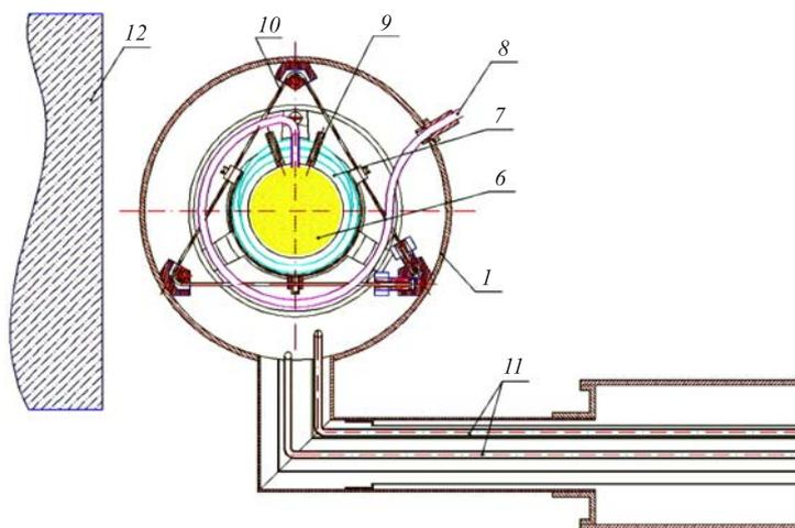
Fig. 2. Front-end of the irradiation rig, elevation through central plane of the sample. 1 — cylindrical shell of the chamber; 6 — aluminium foam filled with solid methane; 7 — coils of copper tube; 8 — steel tube for filling and evacuation gases; 9 — pockets for temperature sensors; 10 — steel string suspender of the sample chamber; 11 — helium pipes inside an evacuated 3-m-long tube; 12 — reactor
