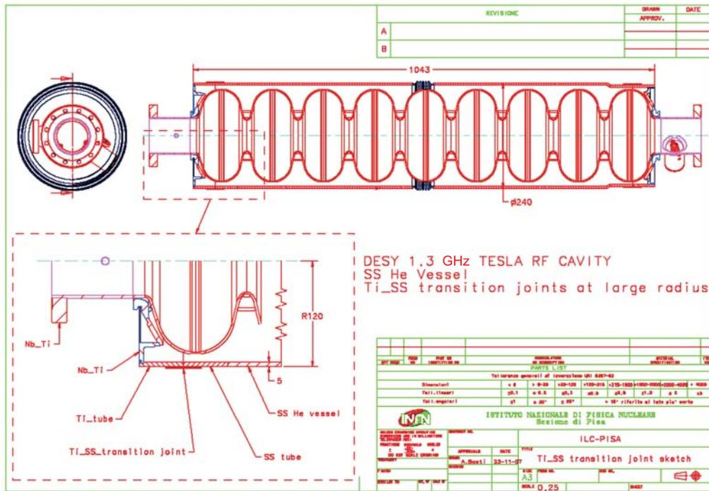
Fig. 3. Technical drawing for a possible construction of a stainless steel He vessel of the TESLA RF cavity. Two bimetallic transition joints (240 mm in diameter) are used for this application
