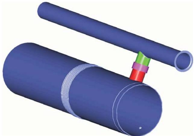
Fig. 2. Sketch of the transition joint (with colours green, pink and red) for the 3rd harmonic cryomodule
