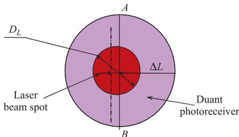
Fig. 5. The laser ray spot position on the duant photoreceiver
