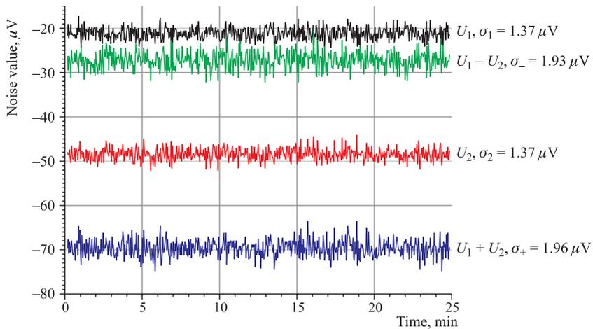
Fig. 2. The noises of the first  $U_1$  and of the second  $U_2$  photosensors; their difference ( $U_1 - U_2$ ) and sum ( $U_1 + U_2$ ). The laser beam is switched off. For  $\sigma$ 's see Figs. 3 and 4
