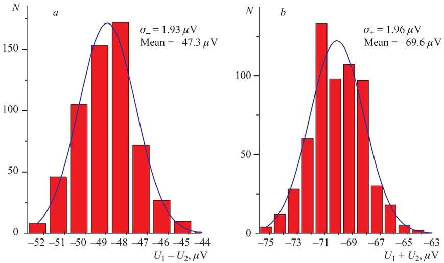
Fig. 4. *a*) Distribution of the difference  $U_1 - U_2$  of noises of the first and second photosensors (25 min measurements). *b*) Distribution of the sum  $U_1 + U_2$  of noises of the first and second photosensors (25 min measurements)
