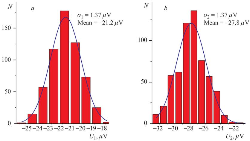
Fig. 3. *a*) Distribution of  $U_1$  — noise of the first photosensor (25 min measurements). *b*) Distribution of  $U_2$  — noise of the second photosensor (25 min measurements)
