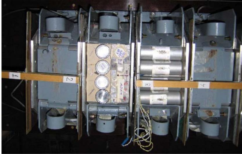
Fig. 2. Top view of the «Energy plus Transmutation» setup with radioactive samples. Beam enters from the left side. The circular samples are assumed to occupy volume of dimensions  $36 \times 36 \times 1.5 \text{ mm}^3$  for the sake of simulation by MCNPX
