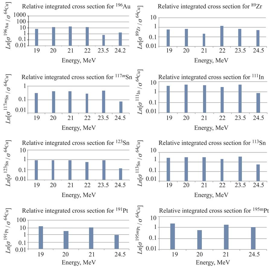
Fig. 3. The distribution of relative integrated cross sections  $[\sigma^x / \sigma^{64\text{Cu}}]$  for some radionuclides at irradiation energies of bremsstrahlung
