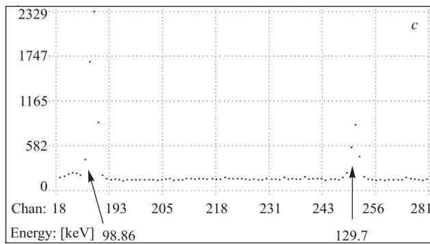
Fig. 2. *a)* A part of gamma spectrum of the irradiated natural pure Sn foil (19.2 mg). There are gamma lines: 158.4 keV for  $^{117m}\text{Sn}$  and 171.3 and 245.3 keV for  $^{111}\text{In}$ . *b)* A part of gamma spectrum of the irradiated enriched  $^{118}\text{Sn}$  (98.5%) foil (29.7 mg). *c)* A part of gamma spectrum of the irradiated natural pure Pt foil (8.6 mg)
