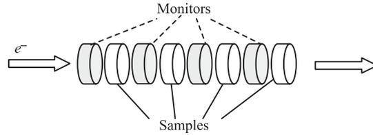
Activity of the irradiated high purity natural platinum, tin and enriched  $^{118}\text{Sn}$  samples and monitors were measured by HPGc detectors of the gamma spectrometer of FLNP, JINR with the energy resolution of 2 keV at gamma lines of 1332 keV for  $^{60}\text{Co}$  radionuclide.
