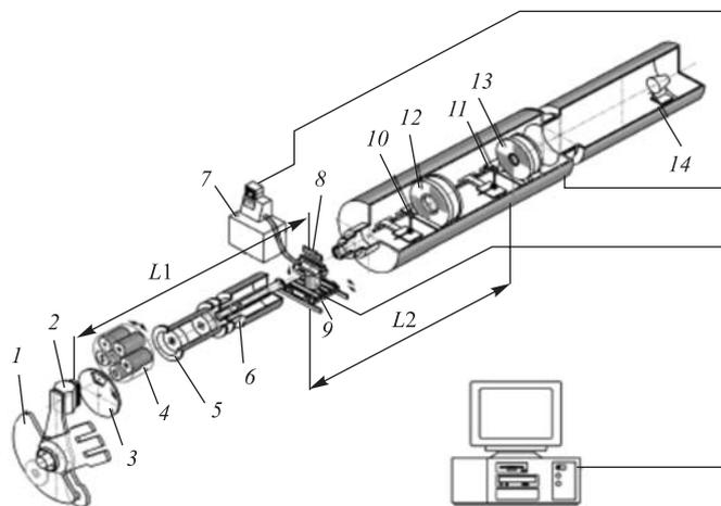
Fig. 1. YUMO SANS TOF spectrometer in function at IBR-2 reactor [1]: 1 — movable reflector; 2 — moderator/cold moderator; 3 — chopper; 4 — first collimator; 5 — vacuum tube; 6 — second collimator; 7 — liquid bath thermostat; 8, 9 — place for the electromagnet during SANS experiments on magnetic samples; 10, 11 — V, graphite, H<sub>2</sub>O standards; 12 — circular detector of thermal neutrons; 13 — PSD circular detector of thermal neutrons; 14 — detector of direct beam
