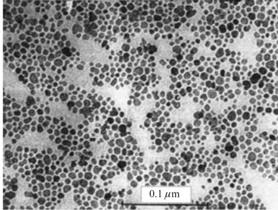
Fig. 4. TEM image of a magnetic fluid sample
