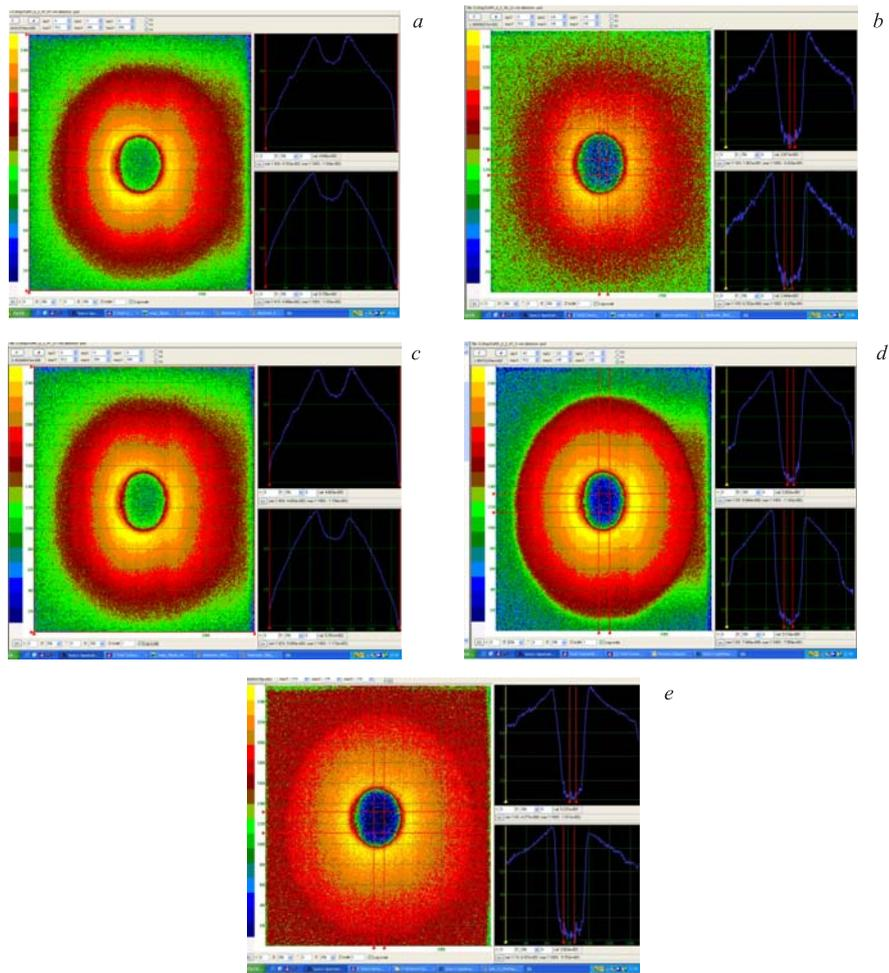
Fig. 6. The 2-dimensional scattering patterns from magnetic elastomer with  $\text{Fe}_3\text{O}_4$  particles in magnetic field of 14 KOe (*a*), 10 KOe (*b*) and without magnetic field (*c*), and from ferrofluid with  $\text{Fe}_3\text{O}_4$  particles in magnetic field of 1 KOe (*d*) and without magnetic field (*e*)
