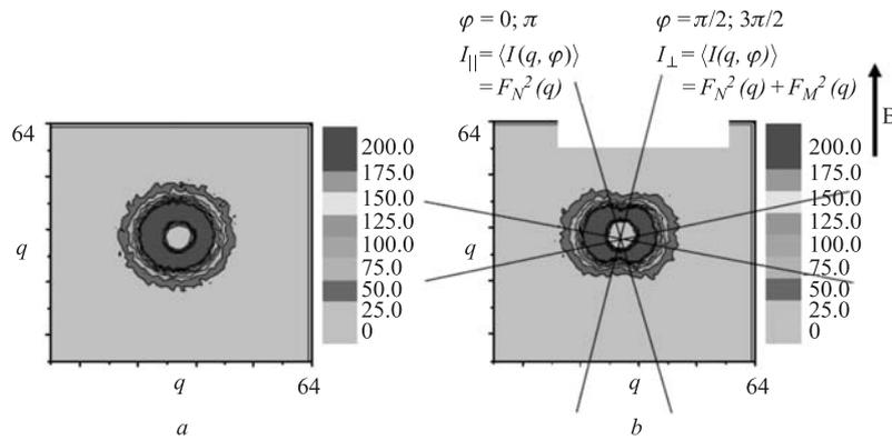
Fig. 5. The 2-dimensional scattering patterns from magnetic sample in absence (a) and presence (b) of external magnetic field. The separation of the nuclear and magnetic scattering contribution for saturated sample is demonstrated
