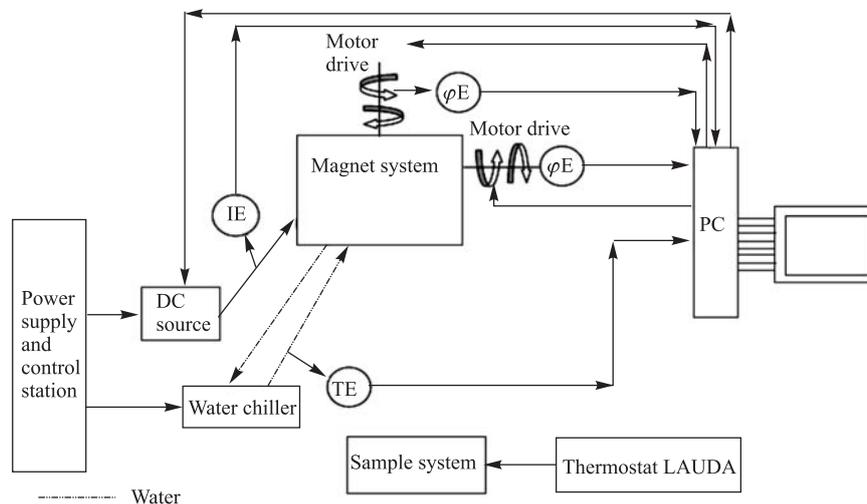
Fig. 3. Block diagram of the whole magnetic system
