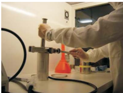
Fig. 31. Tightening procedure of the flanges
