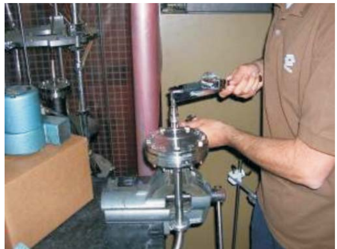
Fig. 10. Leak test during the torque application at LASA
