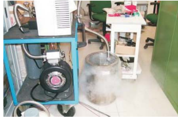
Fig. 27. Helicoflex test in liquid nitrogen
