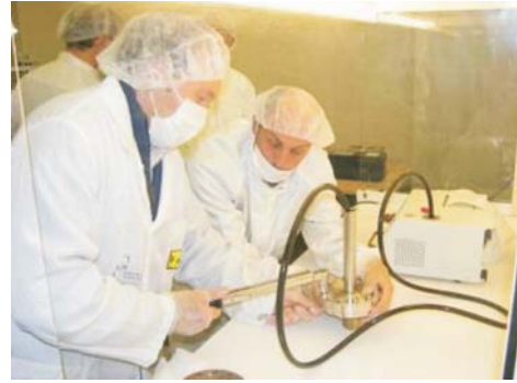
Fig. 15. Flange tightening in the clean room during measurement
