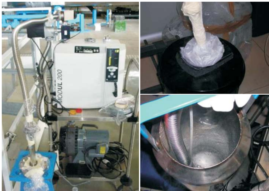
Fig. 9. Leak test measurement of the stainless steel flanges with the Ultra-Flex gasket at 77 K
