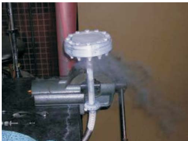
Fig. 12. Ultra-Flex gasket flanges after the dip in nitrogen at LASA
