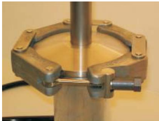
Fig. 25. Photo of the new flange assembly
