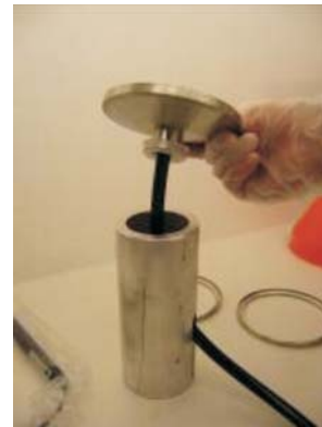
Fig. 30. Particle counter probe inside the bottom flange
