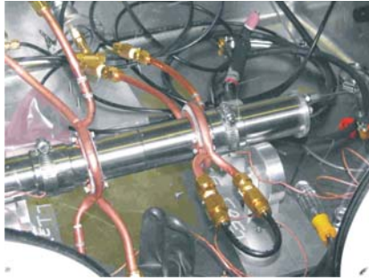
Fig. 7. The heat sinks installed for welding
