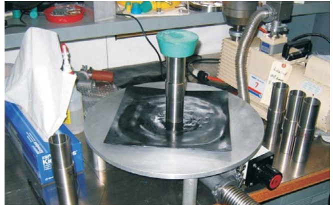
Fig. 3. Initial leak checking at the transition joint at Fermilab
