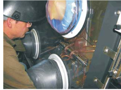
Fig. 8. Welding of the titanium ends of the transition joint test article
