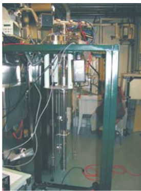
Fig. 10. Transition joint test article mounted on top insert, prior to installation in the A0 VTD
