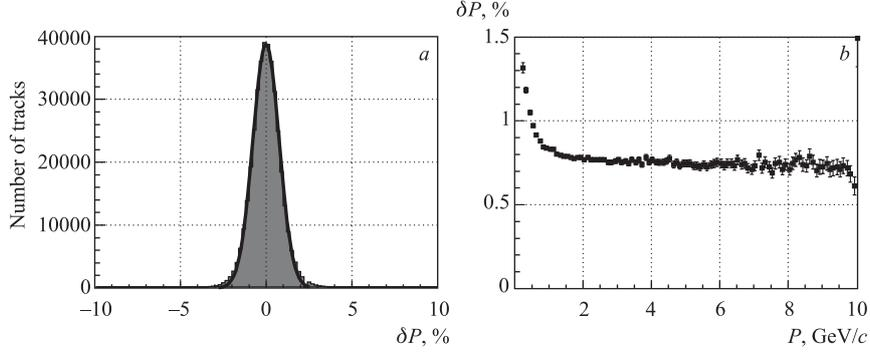
Fig. 4. Momentum resolution  $\delta P \sim 0.79\%$  (a) and momentum resolution vs momentum (b) for CBM STS (7 Si planes)
