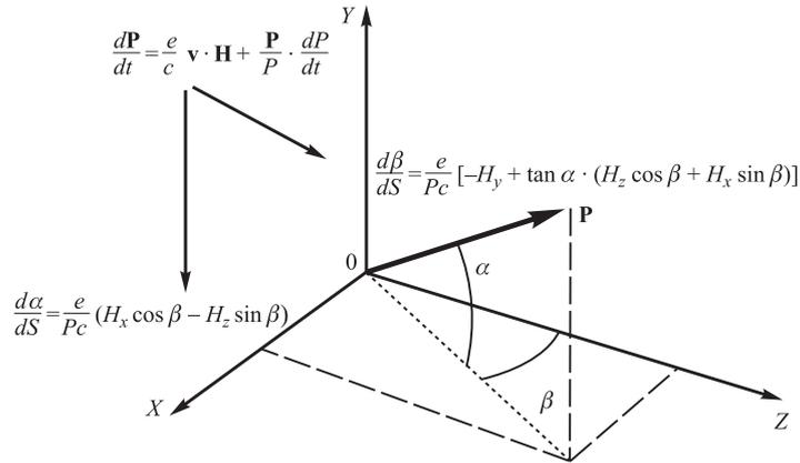
Fig. 1. Coordinate system for ASME method
