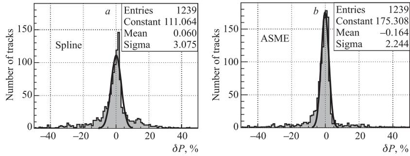
Fig. 7. Momentum resolution for protons: a) spline procedure ( $\delta P \sim 3.08\%$ ); b) ASME ( $\delta P \sim 2.24\%$ )
