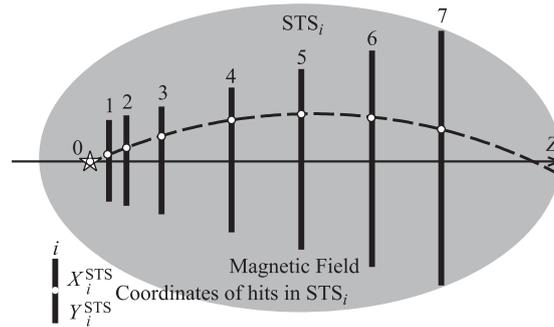
Fig. 2. Scheme of Silicon Tracking Station (STS) of CBM setup
