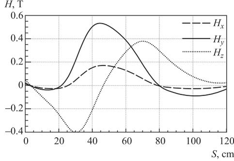
Fig. 6. Magnetic field along the track in MDCs at HADES
