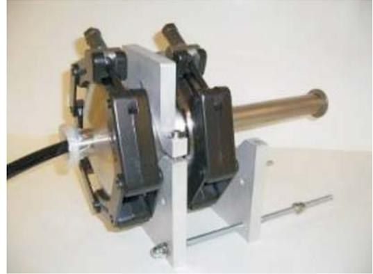
Fig. 15. Sample N1 closed with the Helicoflex gaskets during measurements
