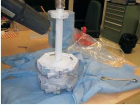
Fig. 20. The sample N1 test during heating with a heat gun
