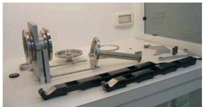
Fig. 13. Set-up for the contamination measurements of sample N1 in the Pisa clean room
