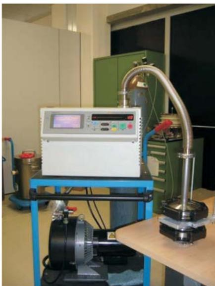
Fig. 18. The sample N1 He-leak test at room temperature
