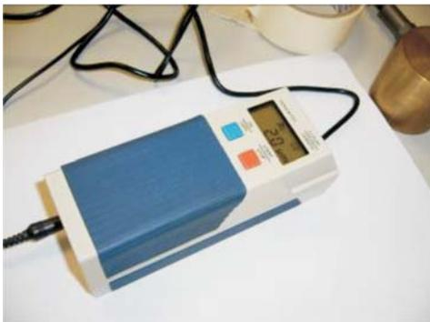
Fig. 6. Mitutoyo surface roughness tester Surftest-211
