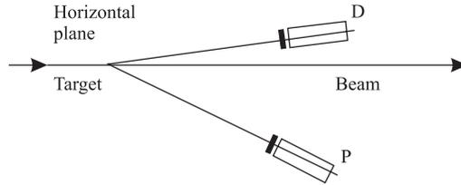
Fig. 1. Schematic view of the experiment. P — proton detector, D — deuteron detector
