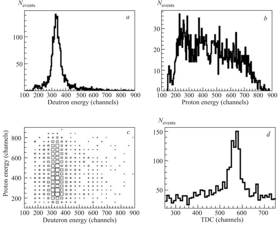
Fig. 4. The results obtained at 2.0 GeV deuteron beam on carbon target: *a*) deuteron energy losses, *b*) proton energy losses, *c*) correlation of proton and deuteron energy losses, *d*) time difference between the signals for deuteron and proton detectors
