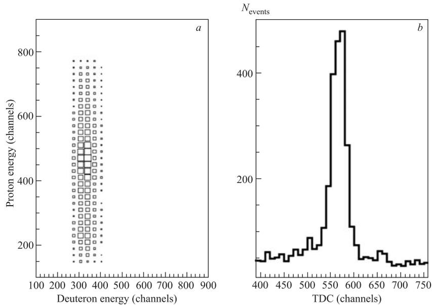
Fig. 3. The selection of the  $dp$ -elastic scattering events by the energy losses correlation (*a*) and time difference (*b*) after applying of the energy losses correlation cut
