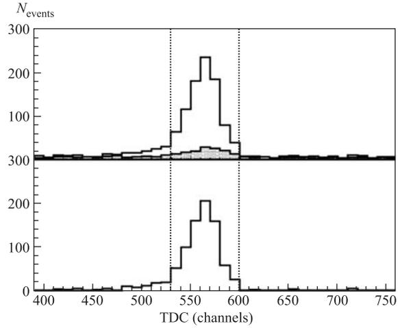
Fig. 6. Time difference distribution for  $dp$ -elastic events obtained from  $\text{CH}_2\text{-C}$  subtraction at a deuteron energy of 1.6 GeV
