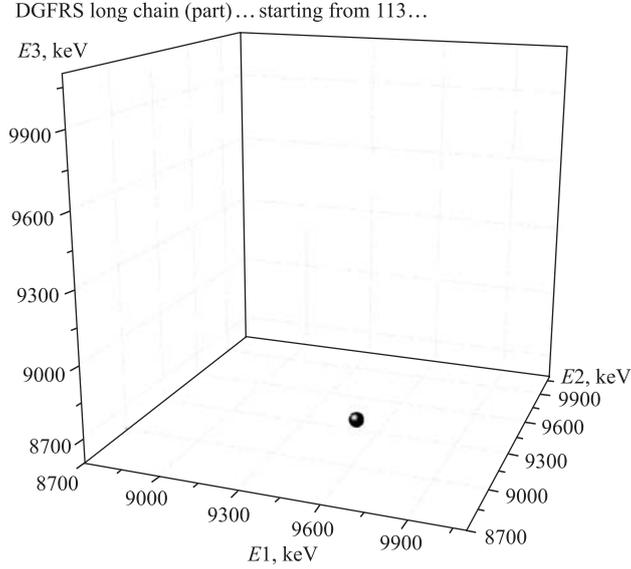
Fig. 3. One decay event from the DGFRS experiment [9] — demonstration of background-free conditions due to application of «active correlations» method
