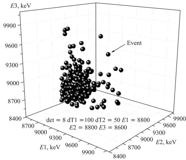
Fig. 2b. 3D picture of  $\alpha$ - $\alpha$ - $\alpha$  group\*. Detected event is indicated by the arrow. Left part — background signals
