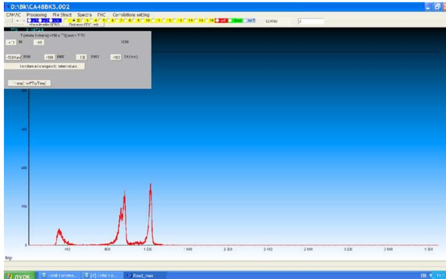
Fig. 2a. Spectrum obtained from the experimental file. Left upper corner — parameters for  $\alpha$ - $\alpha$ - $\alpha$  and  $\alpha$ - $\alpha$ - $\alpha$ -FF correlations search (for a given detector) are shown. (For 16 pairs (top + bottom) with close to  $4\pi$  geometry — 16 buttons in the upper panel). Bottom button in the panel is one to calculate  $N_R$  parameter after correlation search process is finished
