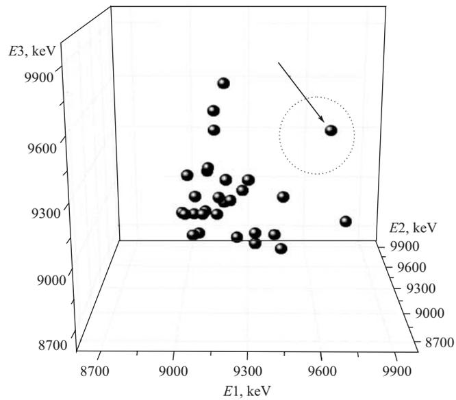
Fig. 2c. 3D picture of  $\alpha$ - $\alpha$ - $\alpha$  group. Detected event is indicated by the arrow. Left part — background signals. *For chain: 9644 keV  $\rightarrow$  8935  $\rightarrow$  9549  $\rightarrow$  8817 987671.312 64.812 6.562 815.625*
