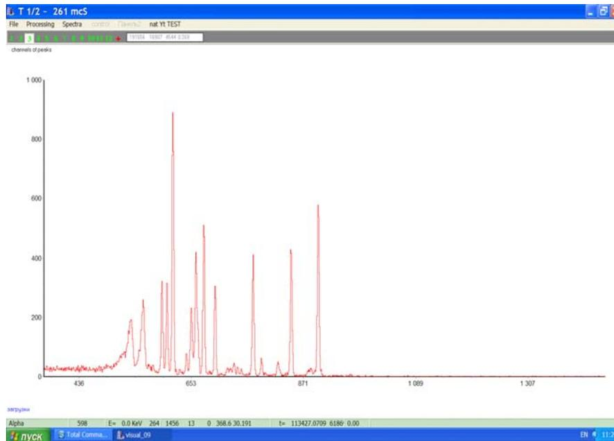
Fig. 6a. Spectrum from  $^{nat}\text{Yt} + {}^{48}\text{Ca} \rightarrow \text{Th}^*$  reaction. Peak under interest is in the right-hand position in the spectrum ( $^{217}\text{Th}$  isotope). Rough estimate value of T1/2 is in the Code form caption (left-upper)
