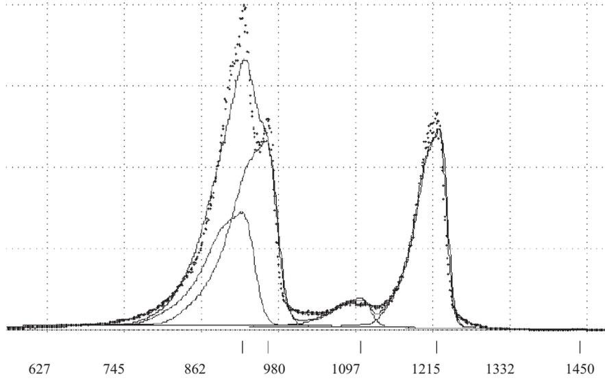
Fig. 5. Measured spectrum (dots) and different peaks (line) according to VMRIA processing from  $^{243}\text{Am} + ^{48}\text{Ca}$  reaction
