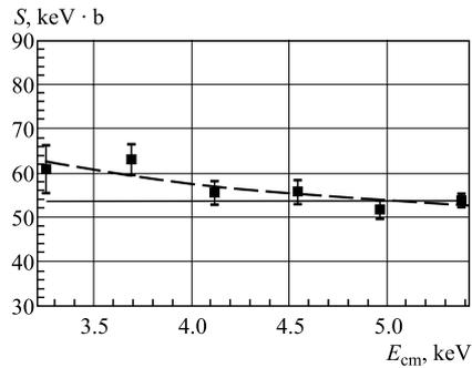
Fig. 8. The astrophysical  $S$ -factor as a function of  $dd$ -reaction energy collision in  $TiD_2$  target. The filled squares are the experimental data, solid line — calculated  $S$ -factor for the «bare» deuterons (Eq. (14)), dashed line — calculated  $S$ -factor for the  $dd$  reactions obtained by using Eqs. (8), (10) and (14) for  $U_e(TiD_2) = 125 \text{ eV}$
