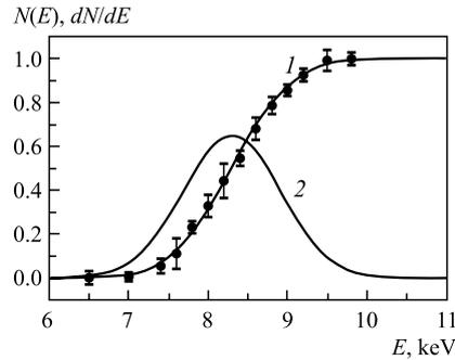
Fig. 3. Energy spectra of deuterons incident on the target: 1 — integral spectrum, 2 — differential
