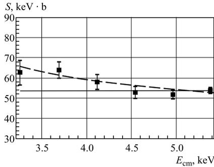
Fig. 7. The astrophysical  $S$ -factor as a function of  $dd$ -reaction energy collision in  $ZrD_2$  target. The filled squares are the experimental data (Eq. (13)), solid line — calculated  $S$ -factor for the «bare» deuterons (Eq. (14)), dashed line — calculated  $S$ -factor for the  $dd$  reactions obtained by using Eqs. (8), (10) and (14), with  $U_e(ZrD_2) = 157 \text{ eV}$
