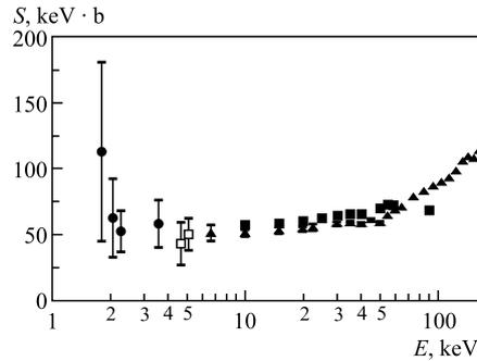
Fig. 4. Values of astrophysical  $S$ -factor for  $d(d, n)^3\text{He}$  reaction obtained in experiments with targets of  $\text{CD}_2$  at different collision energies of deuterons. Filled circles and open squares — experimental values of  $S$ -factor measured in experiments using  $Z$ -pinch technology [32, 33] and Pulsed Hall Accelerator [34, 36], respectively. Filled squares and triangles — data from [42] and [43], respectively
