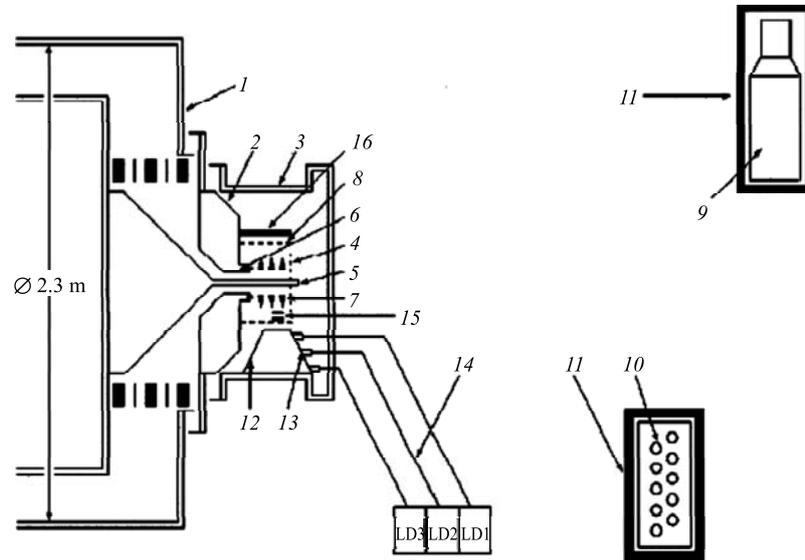
Fig. 1. Scheme of experimental setup: 1 – high-current generator; 2 – accelerator load unit; 3 – measuring chamber; 4 – grid cathode; 5 – reverse-current conductor; 6 – supersonic Laval nozzle; 7 – liner; 8 – current-intercepting rods; 9 – scintillation detector (D1); 10 – thermal-neutron detector (D2); 11 – Pb protective shield; 12 – light cone; 13 – collimators; 14 – fibers; 15 –  $dB/dt$  magnetic probes; 16 – deuterated polyethylene target
