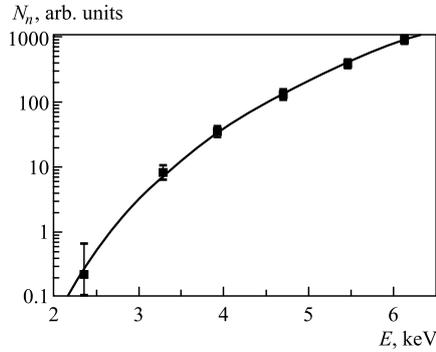
Fig. 5. Neutron yield of the  $dd$  reaction as a function of the deuteron collision energy in the experiment with the  $D_2O$  target. Solid line — calculated neutron yield, filled squares are the experimental data
