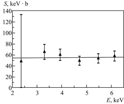
Fig. 6. The astrophysical  $S$ -factor of the  $dd$  reaction as a function of the deuteron collision energy for  $D_2O$  target. The filled triangles are the experimental data; solid line — approximation of the  $S$ -factor for the «bare» deuterons by the linear function  $S_b(E) = S_b(0) + aE$
