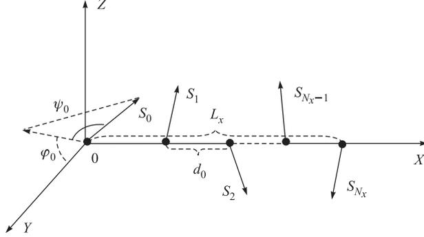
Fig. 1. A stable 1D spatial spin chain with random interactions and length  $L_x = d_0 N_x$ , where  $d_0$  is the distance between nearest neighboring spins,  $N_x$  designates the number of spins in the chain. The spherical angles  $\varphi_0$  and  $\psi_0$  describe the spatial orientation of  $\mathbf{S}_0$  spin, the pair of angles  $(\varphi_i, \psi_i)$  defines the spatial orientation of  $\mathbf{S}_i$  spin
