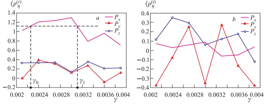
Fig. 5. *a*) Curves of the real part of polarizations are shown on different coordinates ( $x, y, z$ ) after averaging on spin-chains ensemble and on fractal structures. The usual equation of Clausius–Mossotti (2) (without consideration of relaxation effects) for two values of external field ( $\gamma_0, \gamma_1$ ) has catastrophes (plot (*a*)). *b*) Curves of the imaginary part of polarizations are shown after the full averaging by spin-chains ensemble and fractal structures
