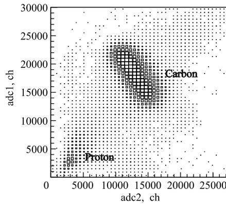
Fig. 5. The signal amplitudes correlation for one of the scintillation detectors of the hodoscope
