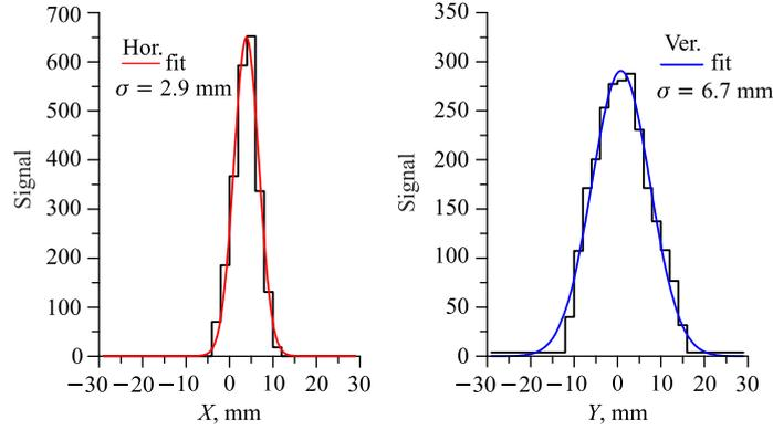
Fig. 4. The  $X$ - (left) and  $Y$ - (right) coordinate beam profile at the focus F5. The lines are the same as in Fig. 7
