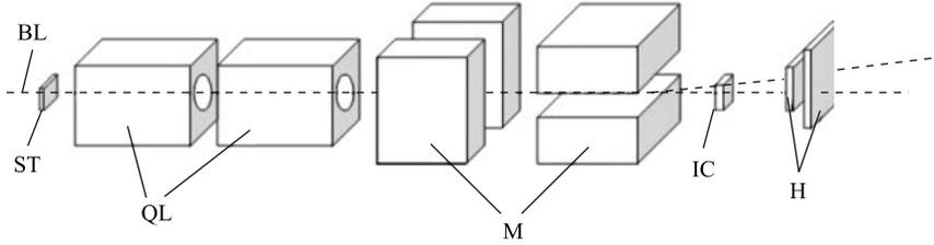
Fig. 2. The layout of the experiment. BL is the optical axis of the 6V beamline, QL and M are the quadrupole and dipole magnets, respectively. IC is the coordinate ionization chamber, ST is the start scintillation counter, H are the two planes of the scintillation counters hodoscopes
