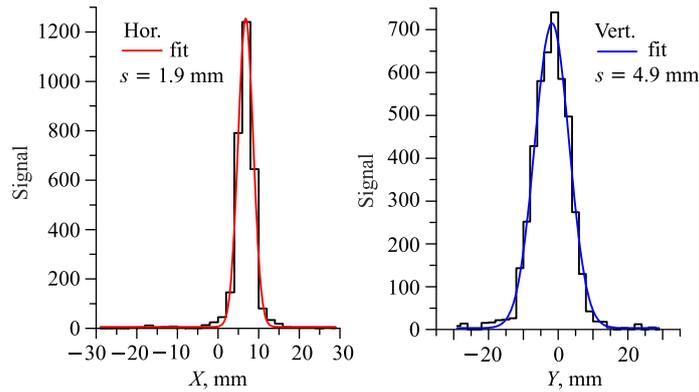
Fig. 3. The X- (left) and Y- (right) coordinate beam profile at the focus F4. The lines are the results of the Gaussian fit
