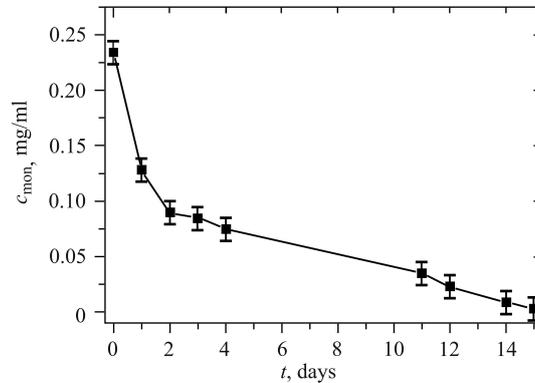
Fig. 4. Evolution of  $C_{60}$  monomer concentration in  $C_{60}/NMP$
