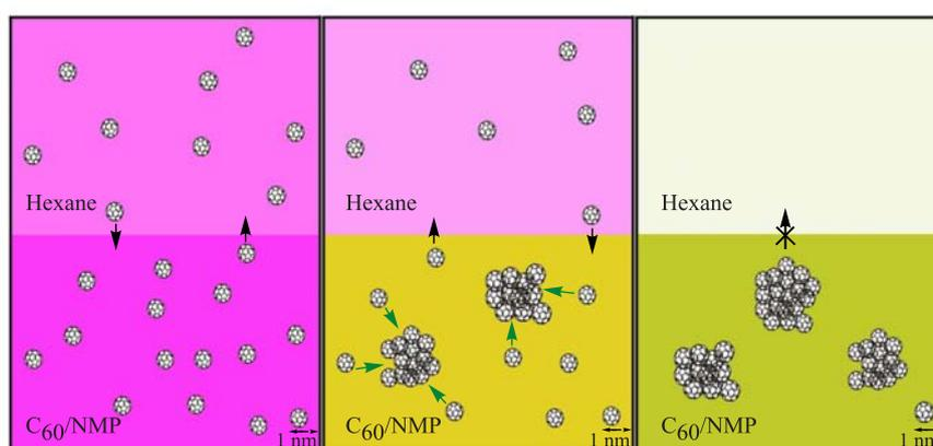
Fig. 3. Representation of extraction of fullerene into molecular solution in hexane from  $C_{60}$ /NMP at different stages of the evolution of solution
