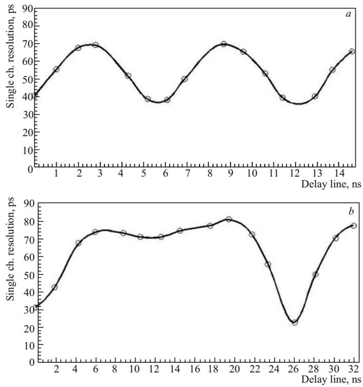
Fig. 7. Jitter in time difference between two channels measured as a function of time delay of one input signal relative to the other one: a) MTDC64; b) TRB HPTDC
