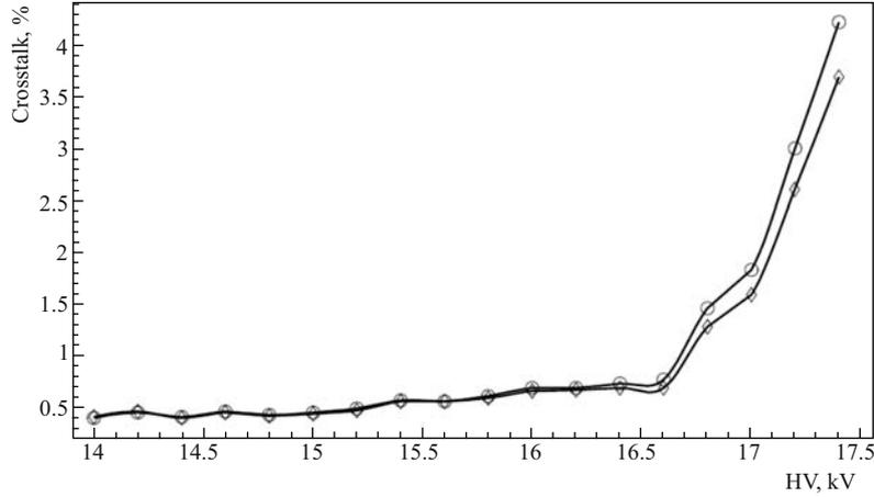
Fig. 10. Fraction of events in which one of adjacent strips located on the left and right sides from the fired strip shows the crosstalk signal
