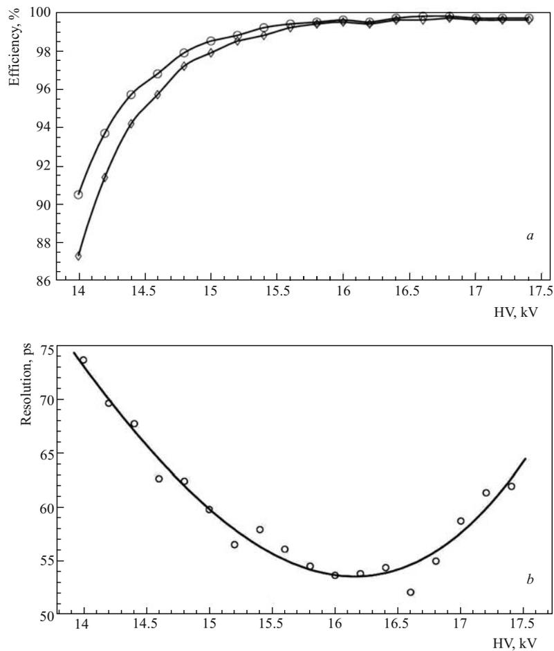
Fig. 9. Efficiency (a) and resolution (b) versus HV for case when TOT signal was digitized by the LeCroy 2228A module. Efficiency is shown for each of the two ends of a strip. The resolution is for the time averaged over the time from two opposite ends
