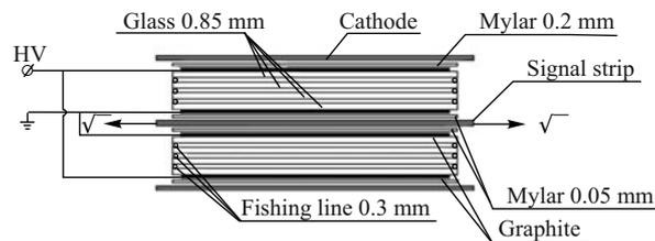
Fig. 1. Schematic cross section of the six-gap MRPC
