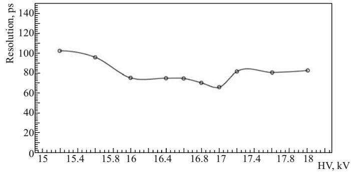
Fig. 6. Time resolution of ten-gap MRPS as a function of high voltage in the case when TRB FEE and HPTDC were used
