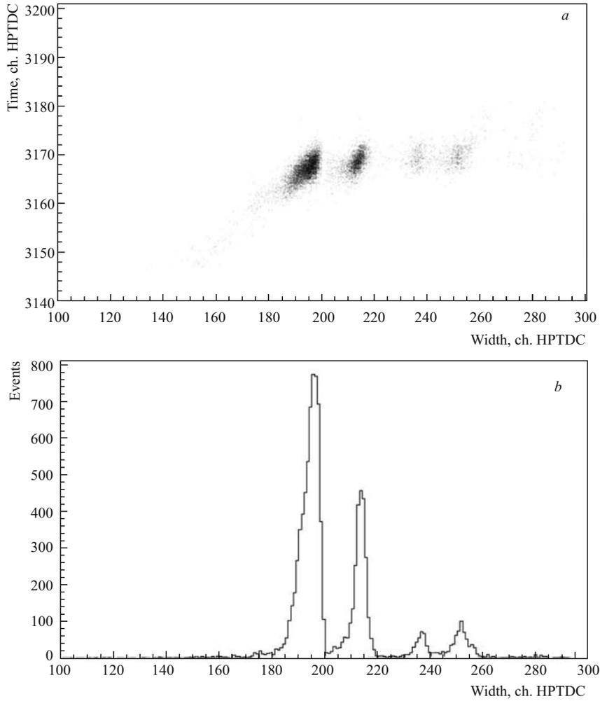
Fig. 3. *a*) Time–width plot for the TOT pulse; *b*) distribution of the TOT signal width. Six-gap MRPC with the ALICE TOF FEE. No matching between strip impedance and the FEE input resistivity
