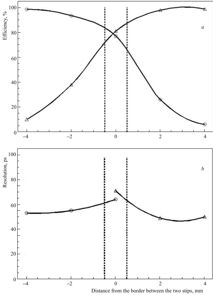
Fig. 11. Changes of efficiency (a) and time resolution (b) near the border between two adjacent strips
