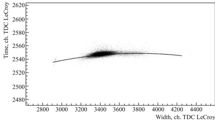
Fig. 8. An example of the time–width correlation. The solid curve is the result of approximation with a polynomial function. Ten-gap MRPC, TOT signals were digitized by the LeCroy 2228A module
