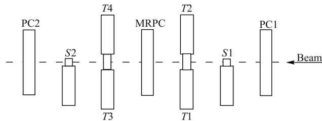
Fig. 2. Sketch of experimental test setup:  $S1, S2$  — beam counters;  $T1, T2$  and  $T3, T4$  — timing counters; RPC — tested chamber; PC1, PC2 — two-coordinate proportional chambers
