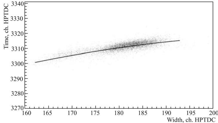
Fig. 4. The time–width correlation plot for six-gap MRPC with the ALICE FEE. All ends of strips are terminated with  $25\ \Omega$  resistors. The solid curve is a polynomial approximation of the data
