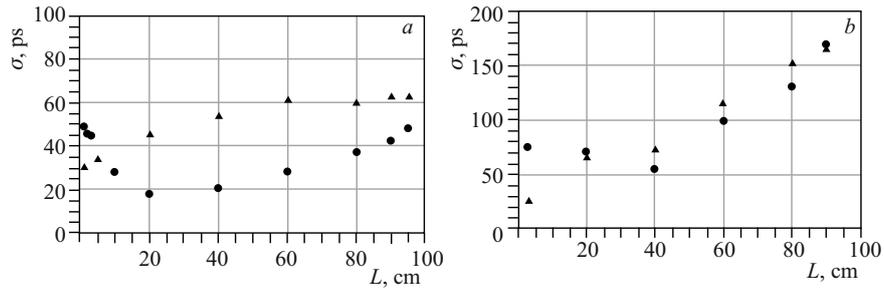
Fig. 4. Accuracy (r.m.s.) of the determination of the longitudinal coordinate along a  $2$  m long straw for incomplete matching. Filled circles — the gas mixture pressure is  $1$  bar and gas gain is  $\sim 7 \cdot 10^4$  (anode voltage is  $1.95$  kV). Filled triangle — the gas pressure is  $3$  bar and the anode voltage is  $3.05$  kV. The matching impedance for each straw end is  $300\ \Omega$ . *a*)  $^{55}\text{Fe}$  source; *b*)  $^{106}\text{Ru}$  source
