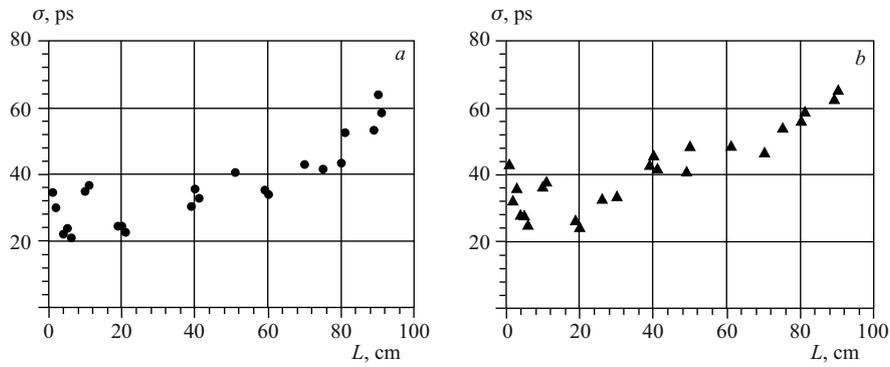
Fig. 6. Spatial resolution along one half of a straw for registering electrons from  $^{106}\text{Ru}$  source. *a)* The gas mixture pressure is 1 bar and the gas gain is  $\sim 7 \cdot 10^4$ . *b)* The gas mixture pressure is 3 bar, the anode voltage is 3.05 kV
