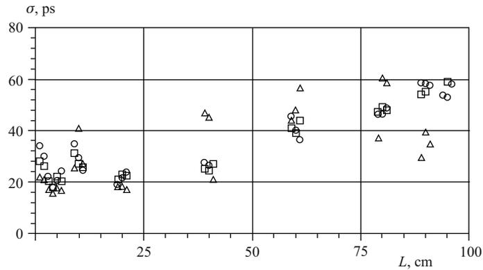
Fig. 5. Spatial resolution along one half of a straw for registering gammas from  $^{55}\text{Fe}$  gamma-ray source. The gas mixture pressure is 1 bar and the gas gain is  $\sim 7 \cdot 10^4$ .  $T_t$  and  $T_b$  levels are 0.2 and 0.7 (open circles), 0.05 and 0.8 (open triangles), and 0.1 and 0.6 (open squares), respectively
