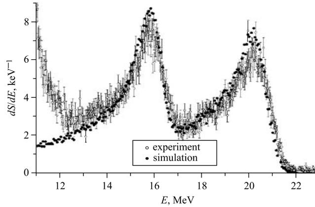
Fig. 3. The energy spectrum of gamma rays  $E_{\gamma 0}$  and  $E_{\gamma 1}$  from reactions (3):  $S$  — partial sum in pulse registration; open circles — measured pulse spectrum vs. pulse amplitudes  $E$ ; filled circles — simulation using GEANT4
