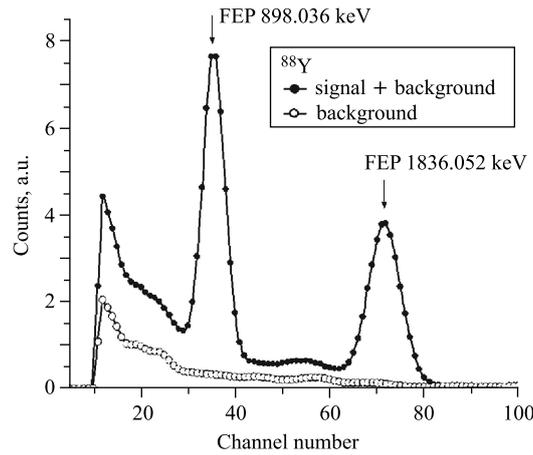
Fig. 2. The energy spectrum for  $^{88}\text{Y}$   $\gamma$ -source: FEP — full-energy peak
