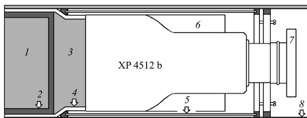
Fig. 1. The gamma detector: 1 — BGO crystal, 2 — plastic scintillator shell, 3 — light-guide, 4 — teflon, 5 — iron magnetic shield, 6 — permalloy magnetic shield, 7 — electronics, 8 — iron casing
