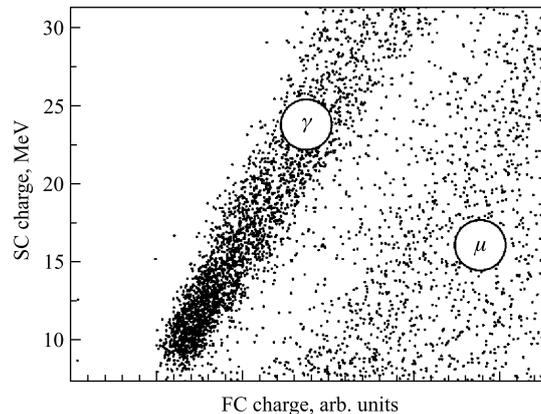
Fig. 5. The two-dimensional FC-SC distribution of the cosmic background (muon and gamma-ray components) obtained with the gamma detector
