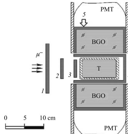
Fig. 6. The experimental setup: 1–4 — muon telescope of plastic counters, 5 — plastic scintillator shell, BGO — scintillation crystal, PMT — photomultiplier, T — target
