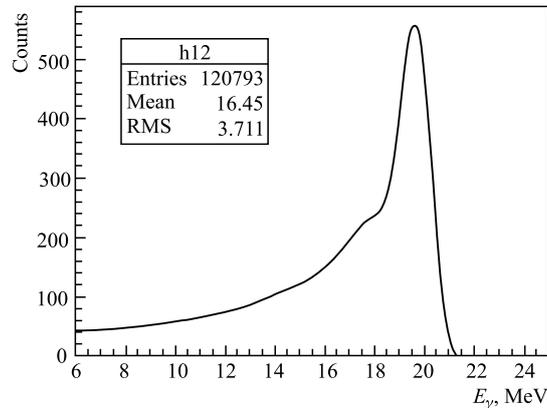
Fig. 9. The calculated gamma spectrometer response function for process (2), which corresponds to gamma line  $E_\gamma = 19.8 \text{ MeV}$
