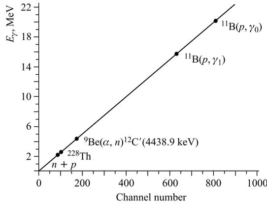
Fig. 4. Data on the energy calibration of the gamma detector
