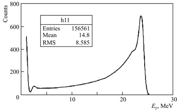
Fig. 7. The calculated response function of the gamma spectrometer for process (1), which corresponds to gamma line  $E_\gamma = 23.8$  MeV
