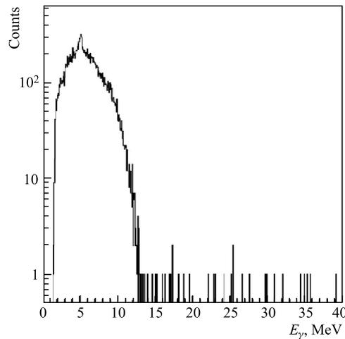
Fig. 8. The experimental gamma-ray energy spectrum registered with the gamma spectrometer
