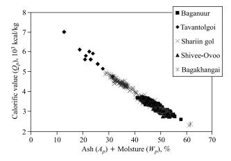
Fig. 6. Comparison of correlations of the calorific value and the sum of ash and moisture content in coal for Baganuur, Tavantolgoi, Shariin gol, Shivee-Ovoo and Bagakhangai coal mines
