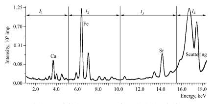
Fig. 2. Four divided X-ray spectrum for coal ash determination
