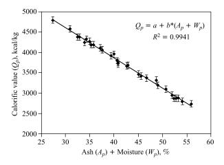
Fig. 5. Correlation between the calorific value and the sum of coal ash and moisture by reference coal samples
