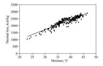
Fig. 4. Relation between the moisture content and thermal loss quantity of coal
