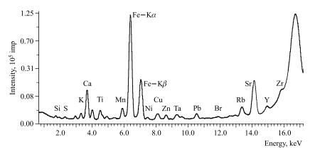
Fig. 1. XRF spectrum of coal sample
