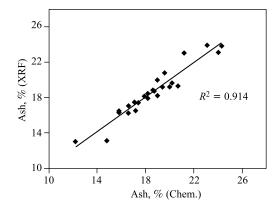
Fig. 3. Comparison of ash contents determined by XRF technique and conventional techniques
