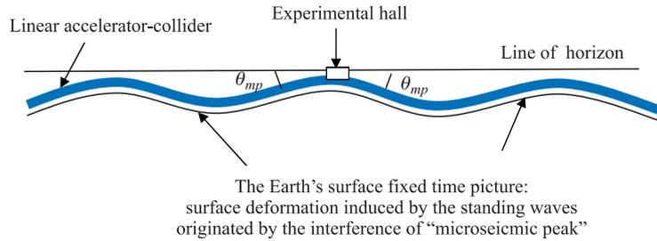
Fig. 10. The accelerator-collider positioning on the Earth's surface deformed by the microseismic peak wave
