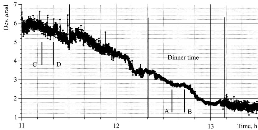
Fig. 5. Earth's surface angular oscillations  $Dev$  ( $\mu rad$ ) of an industrial origin: comparison of the working hours and dinner time data
