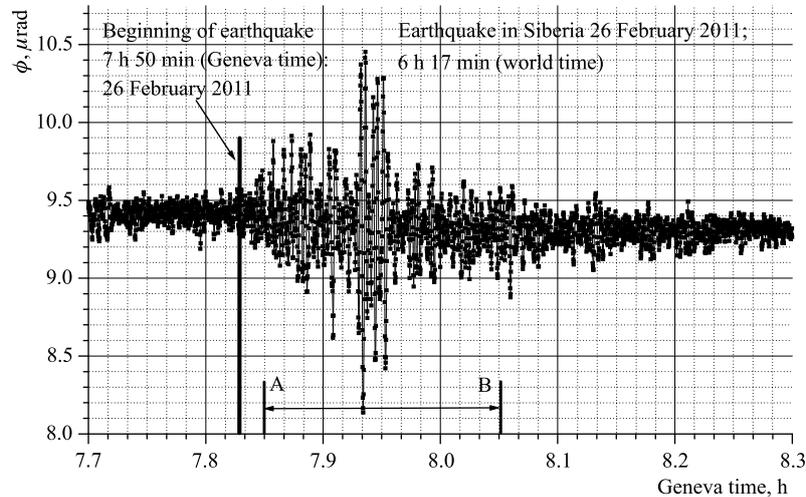
Fig. 2. An Earth's surface inclination angle  $\phi$  ( $\mu\text{rad}$ ) caused by the earthquake in Siberia, registered on 26 February 2011 in Geneva
