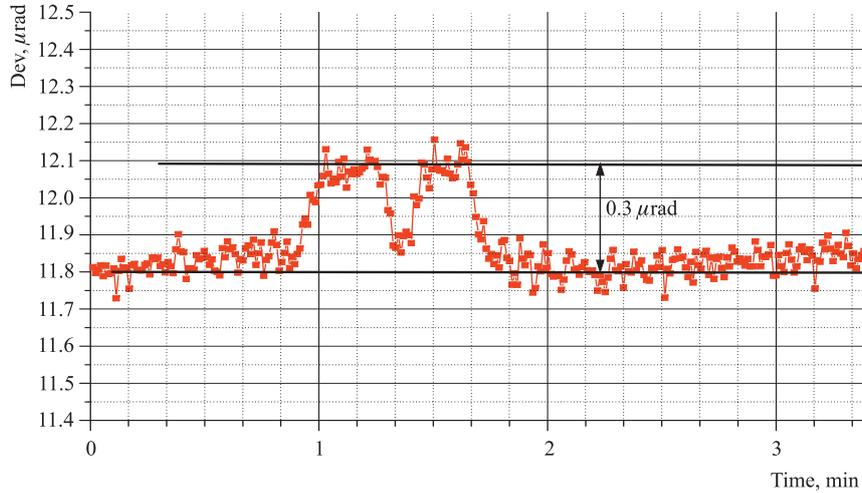
Fig. 7. Concrete floor inclination Dev ( $\mu\text{rad}$ ) due to man presence in 3 m distance from the experimental set-up
