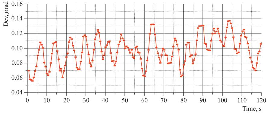
Fig. 8. The seismogram of the Earth's surface angular oscillation at the “microseismic peak” frequency
