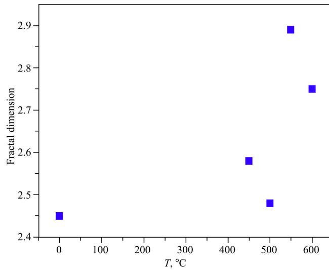
Fig. 8. Fractal dimension variation with heat-treatment temperature of INCOLOY 800HT alloy samples
