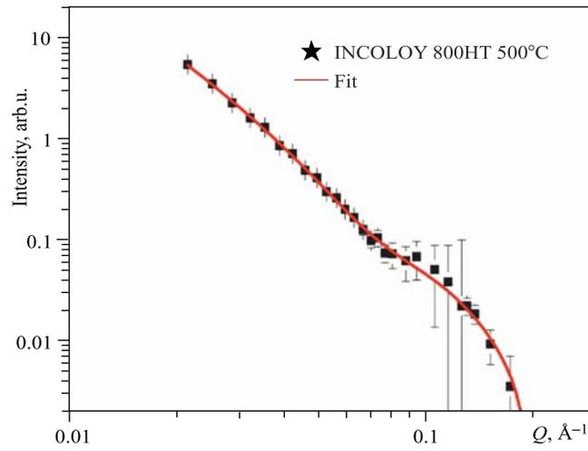
Fig. 4. SANS curve and fit for INCOLOY 800HT with heat treatment (annealing time 60 days) at 500°C
