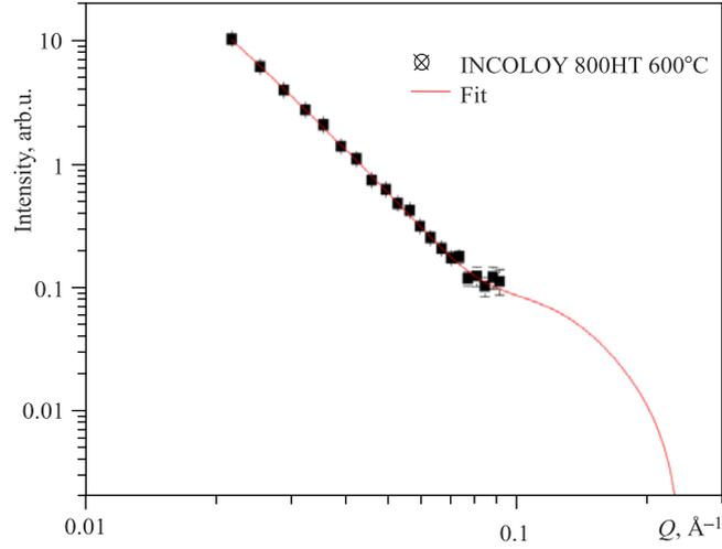
Fig. 6. SANS curve and fit for INCOLOY 800HT with heat treatment (annealing time 60 days) at 600°C
