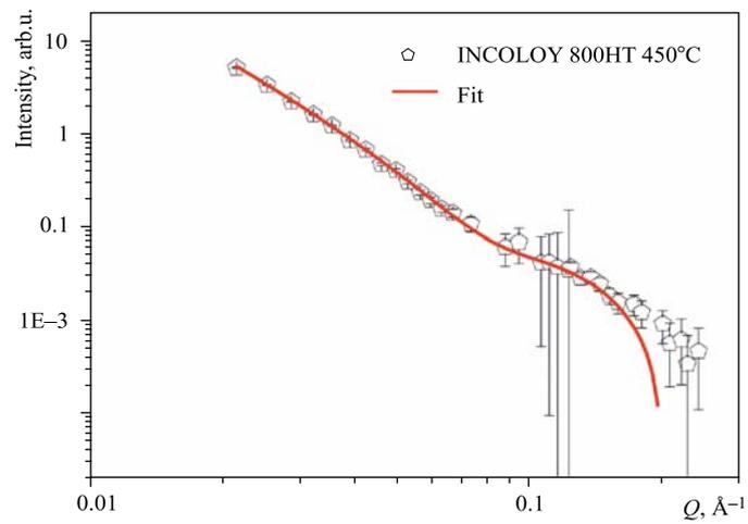
Fig. 3. SANS curve and fit for INCOLOY 800HT with heat treatment (annealing time 60 days) at 450°C
