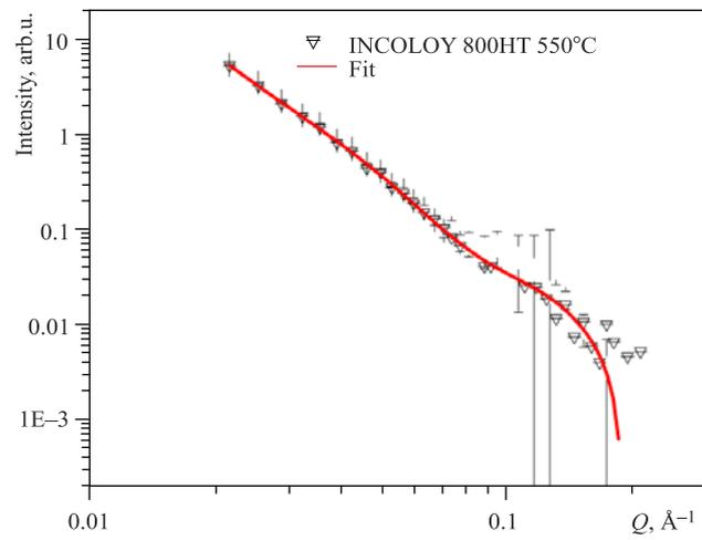
Fig. 5. SANS curve and fit for INCOLOY 800HT with heat treatment (annealing time 60 days) at 550°C
