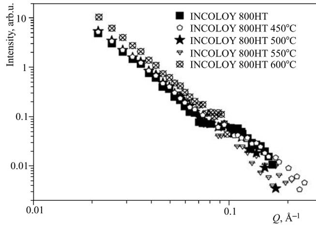
Fig. 1. SANS patterns from INCOLOY 800HT without heat treatment, with heat treatment (annealing time 60 days) at 450°C, 500°C, 550°C, and 600°C
