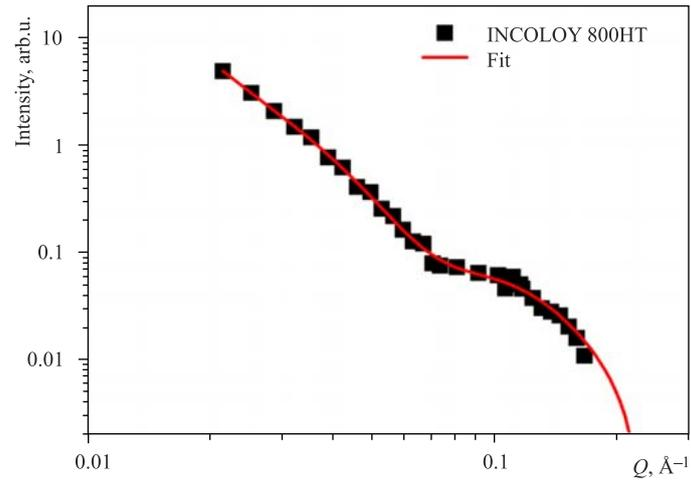
Fig. 2. SANS curve and fit for INCOLOY 800HT without heat treatment
