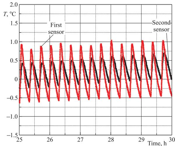
Fig. 4. Time dependence of the stabilized air temperature  $\Delta T$  inside the thermally isolated room with the conditioner HEAT option
