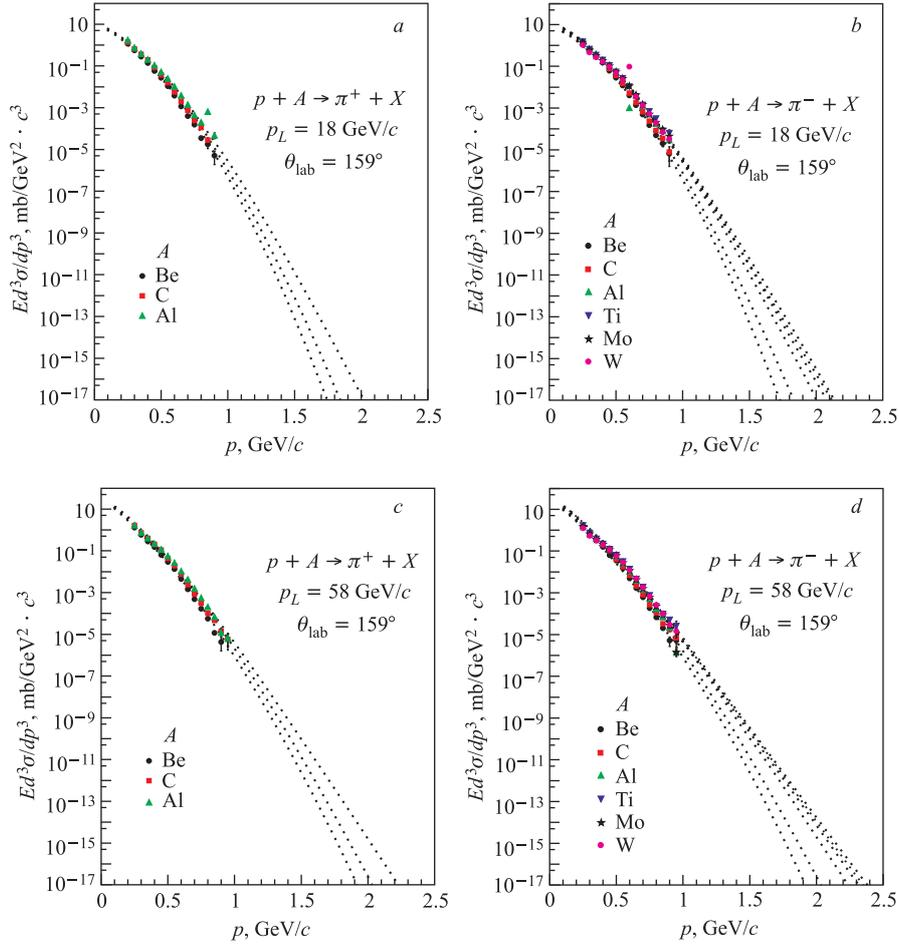
Fig. 3. The dependence of the cross sections of  $\pi^+$  (a, c) and  $\pi^-$  (b, d) pions produced in  $p + A$  collisions on momentum  $p$  at  $p_L = 18, 58 \text{ GeV}/c$  and angle  $\theta_{\text{lab}} = 159^\circ$ . The dotted lines are predictions based on  $z$ -scaling. The experimental data taken from [22] are shown by symbols
