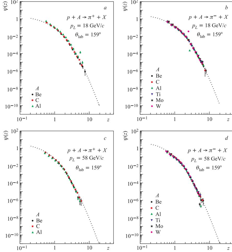
Fig. 2. Scaling function  $\psi(z)$  versus variable  $z$  for  $\pi^+$  (a, c) and  $\pi^-$  (b, d) pions produced in  $p + A$  collisions at  $p_L = 18, 58$  GeV/c and angle  $\theta_{\text{lab}} = 159^\circ$ . The experimental data shown by symbols are taken from [22]. The dotted lines are the results of fitting the experimental data on inclusive momentum spectra taken from [31, 33–35]
