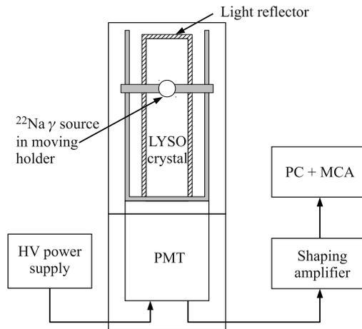
Fig. 2. The block diagram of the setup for measuring the  $30 \times 30 \times 130$  mm LYSO crystal light response uniformity
