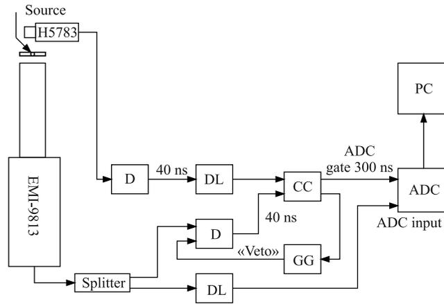
Fig. 1. The block diagram of the setup for measuring the  $30 \times 30 \times 130$  mm LYSO crystal energy resolution
