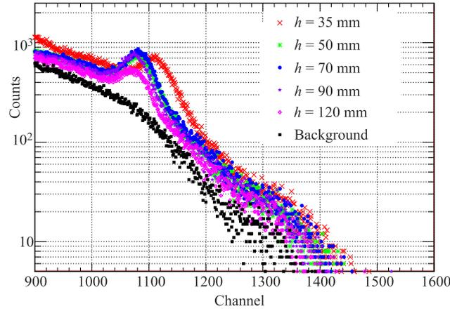
Fig. 10. Pulse height spectra of the  $30 \times 30 \times 130$  mm LYSO crystal irradiated by the  $^{22}\text{Na}$   $\gamma$  source placed at distances of 35, 50, 70, 90 and 120 mm from the PMT cathode (1786 keV full absorption peaks are around channel 1100)
