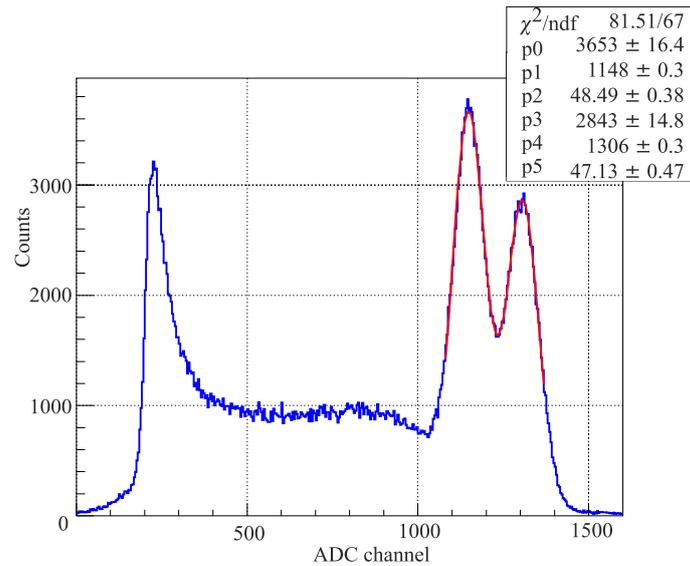
Fig. 7. LYSO spectra due to  $^{60}\text{Co}$  irradiation. Two full absorption peaks corresponding to 1173 and 1333 keV are fitted with the sum of two Gaussians
