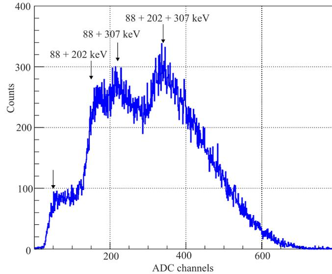
Fig. 12. The  $10 \times 10 \times 10$  mm LYSO crystal spectrum due to intrinsic radioactivity measured with the S8664-1010 series Hamamatsu APD. Four sets of detected gammas are shown in the spectrum by arrows
