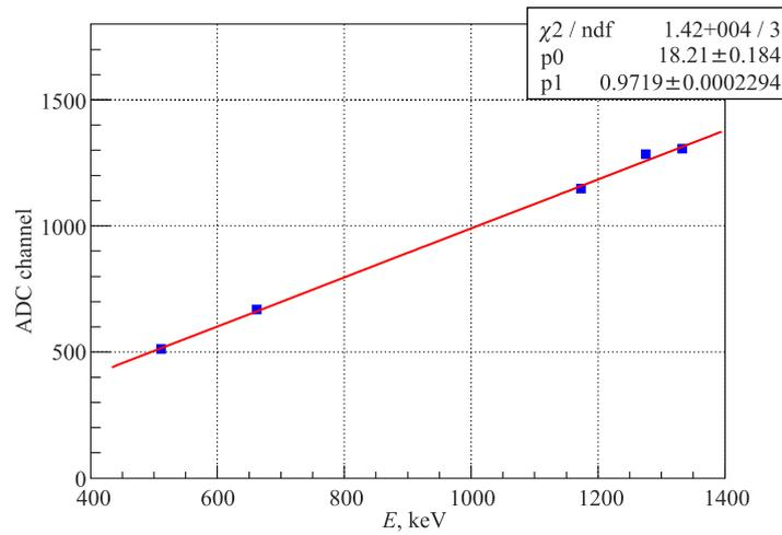
Fig. 9. The  $30 \times 30 \times 130$  mm LYSO crystal energy response linearity in the 511–1333 keV range
