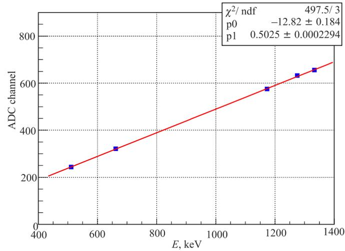
Fig. 15. The  $10 \times 10 \times 10$  mm LYSO crystal energy response linearity in the 511–1333 keV range measured by the S8664-1010 Hamamatsu APD
