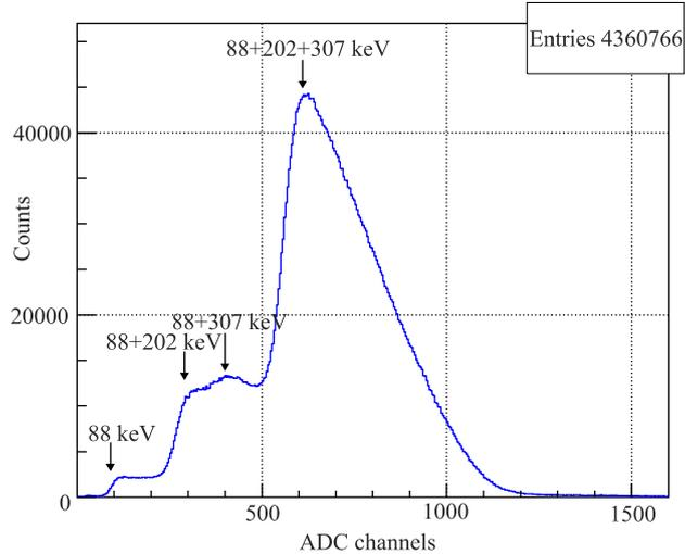
Fig. 4. The  $30 \times 30 \times 130$  mm LYSO crystal spectrum due to intrinsic radioactivity. Four sets of detected gammas are shown in the spectrum by arrows
