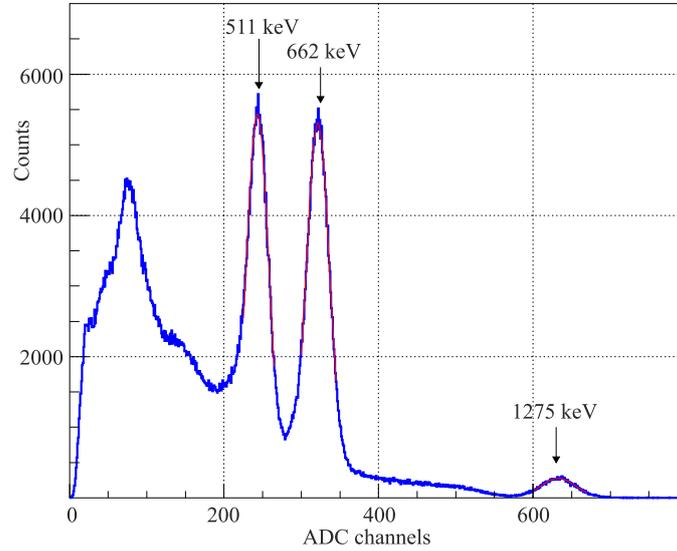
Fig. 13. The  $10 \times 10 \times 10$  mm LYSO crystal spectrum due to intrinsic radioactivity and  $^{22}\text{Na}$  and  $^{137}\text{Cs}$  irradiation. Three full absorption peaks are fitted with Gaussians
