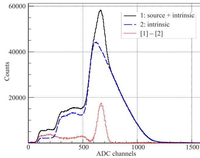
Fig. 6. LYSO spectra due to intrinsic radioactivity and  $^{137}\text{Cs}$  irradiation: total spectrum (solid line), spectrum due to intrinsic radioactivity (dashed line), and spectrum due to  $^{137}\text{Cs}$  irradiation (dotted line)
