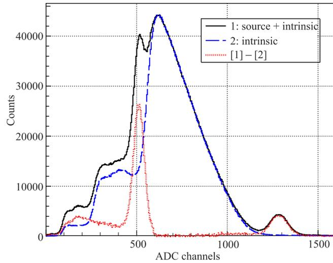
Fig. 5. LYSO spectra due to intrinsic radioactivity and  $^{22}\text{Na}$  irradiation: total spectrum (solid line), spectrum due to intrinsic radioactivity (dashed line), and spectrum due to  $^{22}\text{Na}$  irradiation (dotted line)
