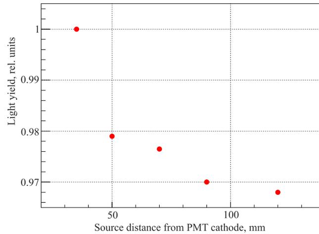
Fig. 11. Longitudinal light response uniformity of the  $30 \times 30 \times 130$  mm LYSO crystal. Nonuniformity does not exceed 3.2% for the  $\gamma$ -source position ranging between 35 and 120 mm on the crystal axis
