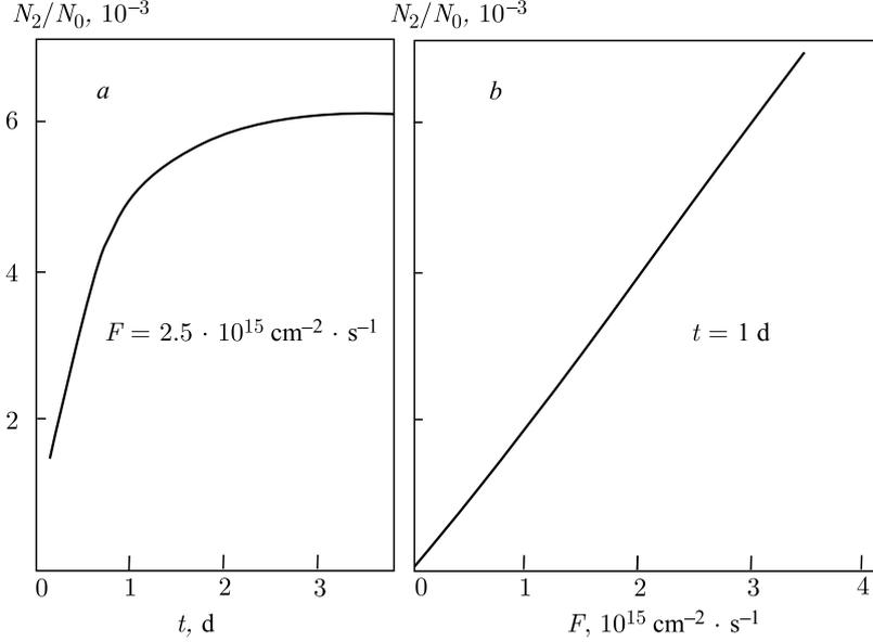
Fig. 1. Calculated number of produced  $^{195m}\text{Pt}$  nuclei as a function of time (a) and of neutron flux (b)
