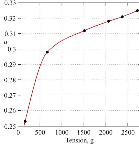
Fig. 3. Dependence of Poisson's ratio on the straw tube tension
