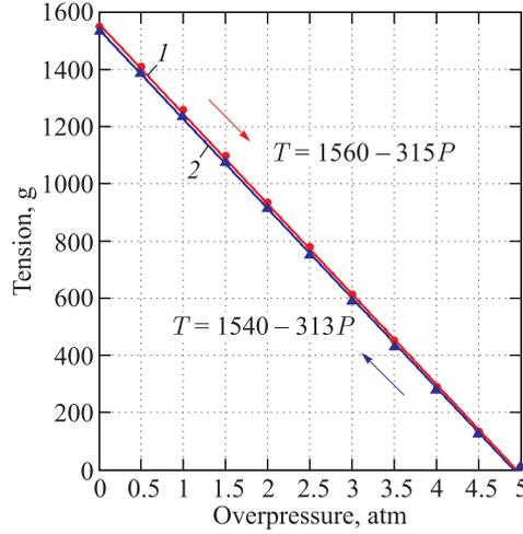
Fig. 2. Straw tension variation under the effect of the internal pressure
