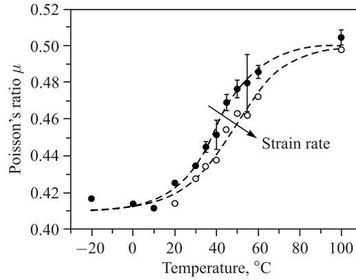
Fig. 4. Dependence of Poisson's ratio on the temperature and deformation rate: ● — deformation rate  $0.003 \text{ s}^{-1}$ , ○ — deformation rate  $0.05 \text{ s}^{-1}$
