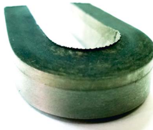
Fig. 7. Bimetal steel–titanium sample after bending test
