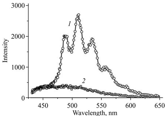
Fig. 3. 1 — photoluminescence of  $\text{UO}_2\text{F}_5^{3-}$  (0.005 M) in  $\text{CsF}$  (42%) +  $\text{H}_2\text{O}$  + luminol ( $10^{-4} \text{ M}$ ); 2 — luminol  $10^{-4} \text{ M}$  in  $\text{CsF}$  (42%) +  $\text{H}_2\text{O}$ ,  $\text{pH} 10.07$ . Excitation by pulsed (10 ns) nitrogen laser. Delay time  $2 \mu\text{s}$ . Gate time  $100 \mu\text{s}$
