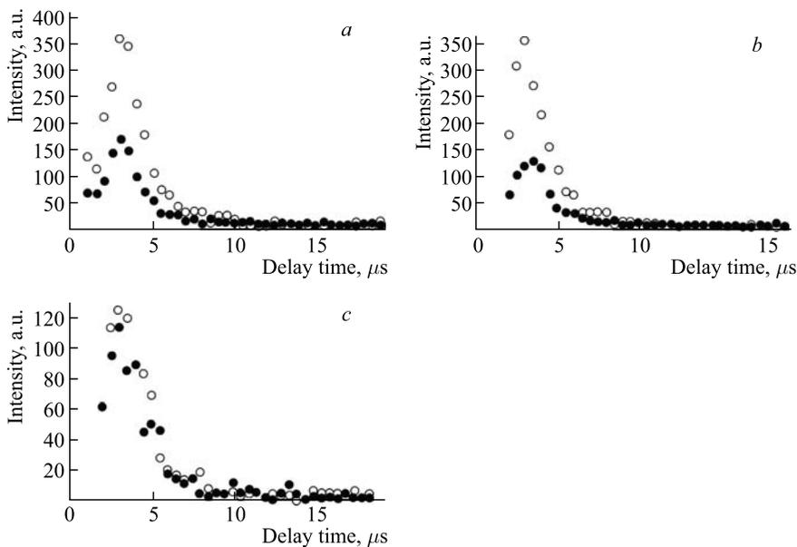
Fig. 4. Kinetics of luminol luminescence at the wavelength 459 nm in 42% solution of CsF in  $\text{H}_2\text{O}$ . pH: 8.19 (*a*), 9.86 (*b*), 11.85 (*c*). Open circles — without uranium, filled circles — 0.009 M of  $\text{UO}_2^{2+}$ . Luminol concentration  $10^{-4}$ . Gate time 1  $\mu\text{s}$
