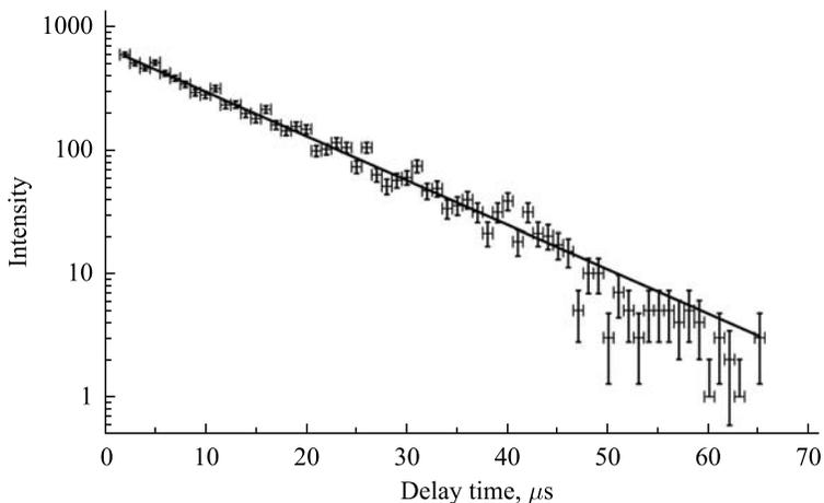
Fig. 2. Photoluminescence of  $\text{UO}_2\text{F}_5^{3-}$  in  $\text{H}_2\text{O} + \text{CsF}$  (42%) solution.  $\text{pH} = 9.0$ . Excitation by nitrogen pulse (10 ns) laser. Registration at  $\lambda = 520 \text{ nm}$ ,  $\delta\lambda = 9 \text{ nm}$ . Gate time  $1 \mu\text{s}$ . 200 laser pulses per channel were made. Laser beam diameter 5 mm, power in laser pulse 15 kW. Luminescence lifetime  $\tau = 12.08 \pm 0.25 \mu\text{s}$
