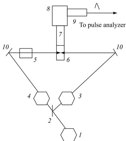
Fig. 8. Scheme of the experimental setup: 1 — nitrogen laser OBB-1010; 2 — beam splitter; 3 — dye laser OBB-1011; 4 — dye laser OBB-1012; 5 — optical delay line OPD-1; 6 — cuvette with solution; 7 — optical fiber; 8 — monochromator DMR-4; 9 — photomultiplier; 10 — mirror
