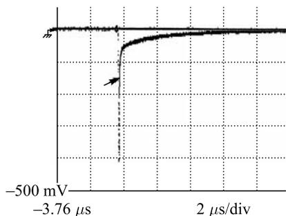
Fig. 1. Time dependence of the uranyl luminescence in a 4.5 M  $H_2SO_4$  solution. Start is a nitrogen laser pulse. The short-lived background luminescence is clearly seen, as well as the relatively long-lived uranyl luminescence. The background luminescence can be significantly suppressed by measuring the luminescence with a delay of several microseconds after laser pulse
