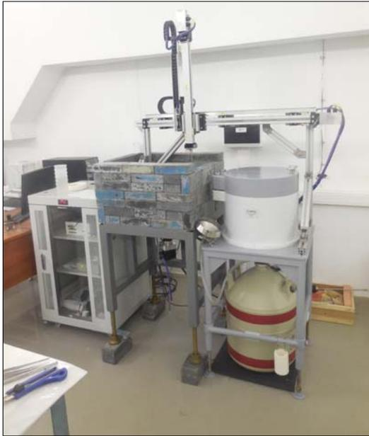
Fig. 6. Automation system for measurement of spectra
