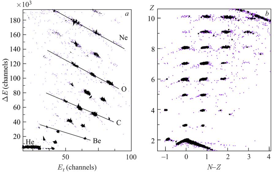
Fig. 1. *a*) Particle identification plot for the products of the  $^{48}\text{Ca} + \text{Ta}$  reaction from  $^4\text{He}$  up to Ne-isotopes.  $\Delta E$  is the energy loss and  $E_r$  is the residual energy. *b*) Identification matrix (product yield versus atomic number  $Z$  and neutron excess  $N-Z$  values) obtained by the so-called  $\Delta E-E$  method
