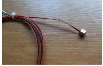
Fig. 3. Tested Pt100 platinum resistance thermometer
