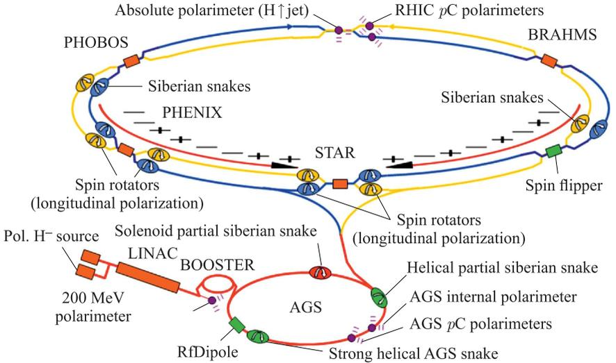
Fig. 1. Polarized  $p + p$  collider at BNL [2]
