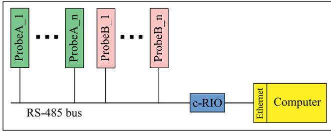
Fig. 4. The schematic view of the prototype dosimetry system for protecting MPD Slow Control electronics from unexpected irradiation
