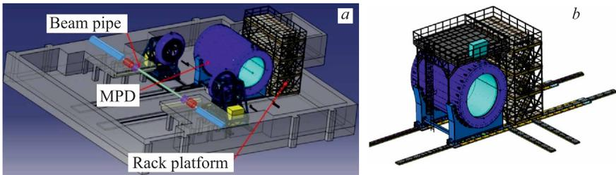
Fig. 1. *a)* Room for the MPD detector; *b)* MPD detectors and platform for the MPD electronic racks [1]
