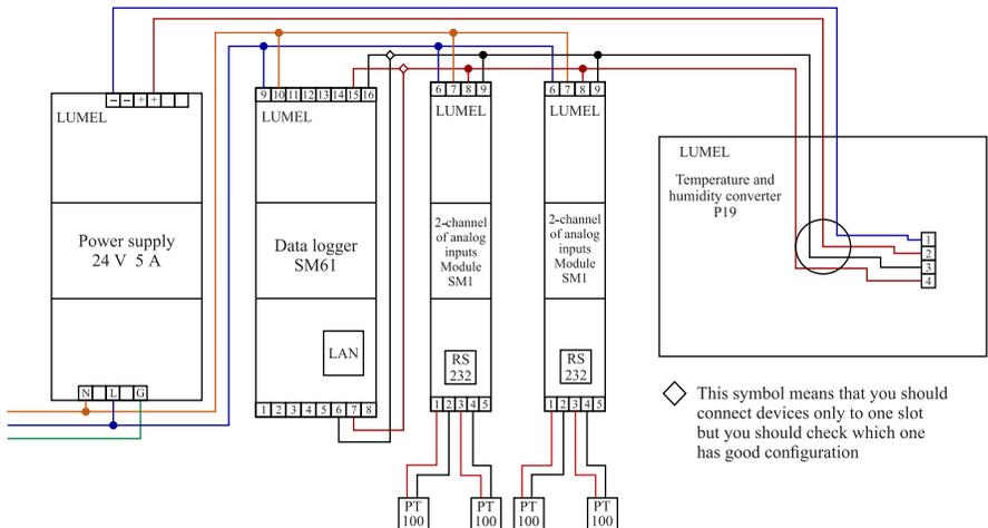
Fig. 1. Schematic diagram of temperature measurement system (TMS)
