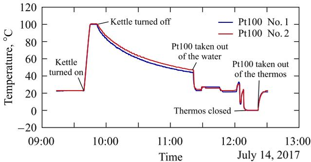
Fig. 4. Periodic scheme of the whole calibration process
