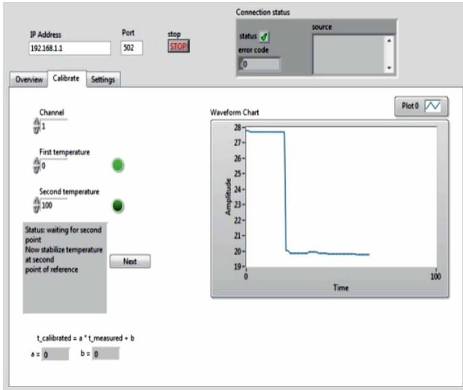
Fig. 3. TMS LabView program — calibration panel
