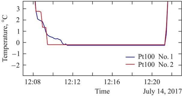
Fig. 5. Calibration at freezing point
