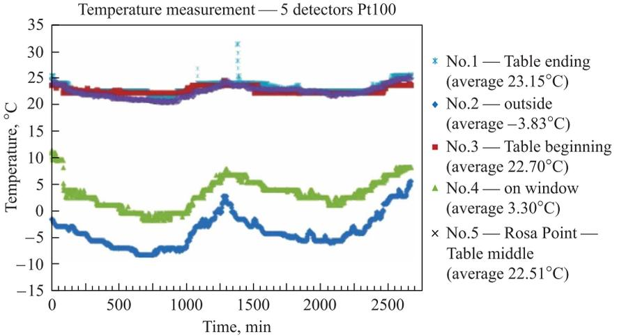
Fig. 7. TMS two-day measurement at 5 points simultaneously. Probes No. 1, 3 and 5 were inside the room, probes No. 2 and 4 — outside the room. Measurement “0” min start point 15.02.2017 15:00
