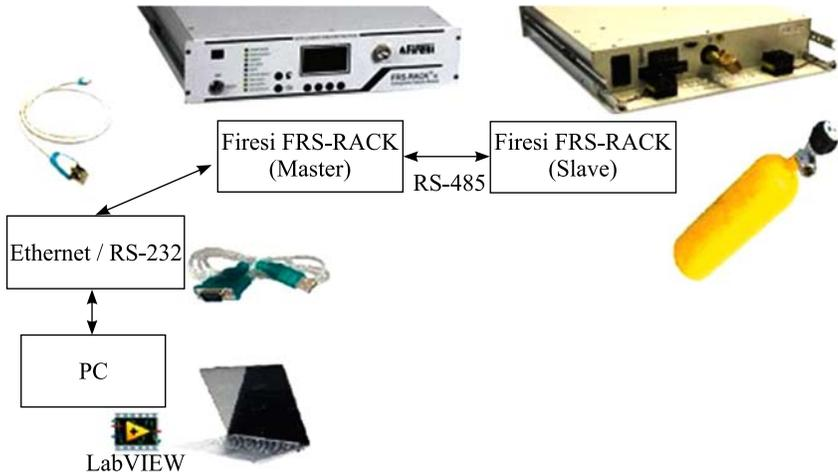
Fig. 1. Structure scheme of the fire extinguishing system [1]
