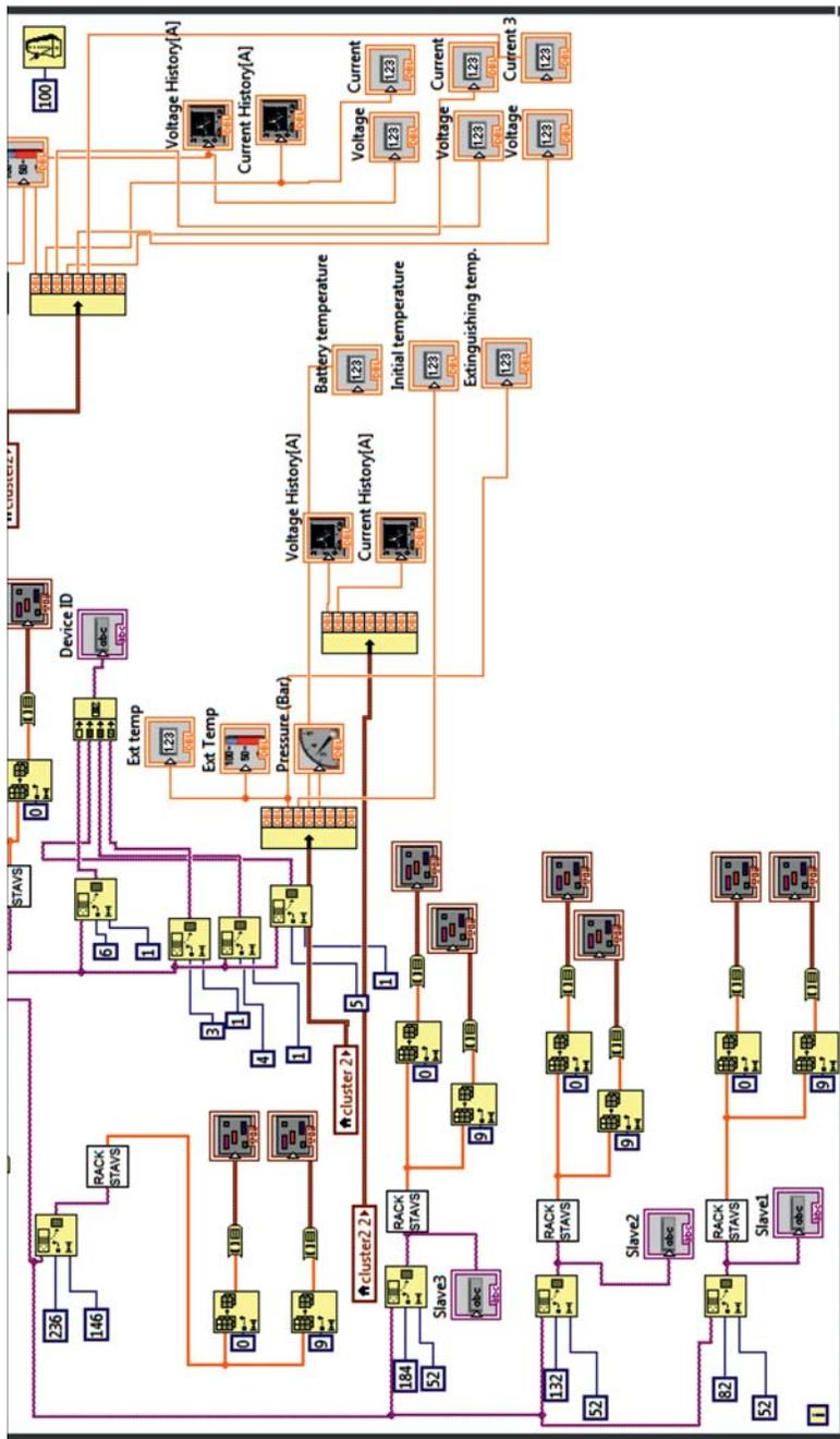
Fig. 6. The second part of main block diagram written in G language using the LabVIEW 2016 environment
