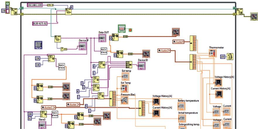
Fig. 5. The first part of the main block diagram written in G language using the LabVIEW 2016 environment
