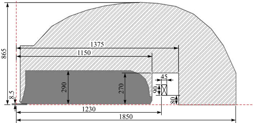
Fig. 2. SC230 magnet yoke and SC coil general dimensions (in mm)
