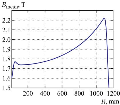
Fig. 3. Average magnetic field along the radius
