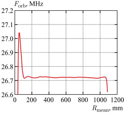
Fig. 5. Orbital frequency against mean radius
