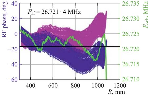
Fig. 10. Phase motion of the beam (blue line — in the convex gap, magenta — in the concave gap of the cavities)
