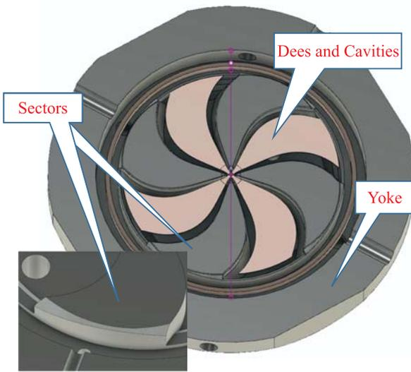
Fig. 1. Layout of the cyclotron's 3D computer model (magnet and accelerating system)
