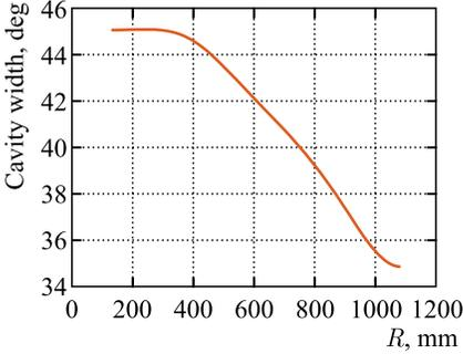
Fig. 8. Azimuthal extension of the cavity (between the middles of acceleration gaps)
