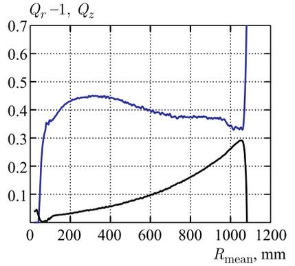
Fig. 6. Vertical and radial betatron tunes in SC230
