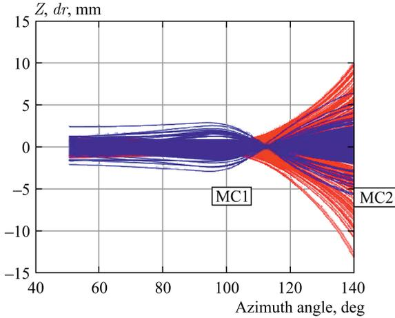
Fig. 11. Beam path through the ES deflector ( $50^\circ$ – $90^\circ$ ). Red lines — horizontal, blue lines — vertical motion. Suitable positions for gradient correctors are marked by MC1, MC2
