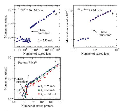
Fig. 8. Dependence of the momentum spread  $(1\sigma)$  on the number of beam particles in the electron-cooled storage rings:  $a)^{238} \mathrm{U}^{92+}$  in the ESR [24],  $b)^{129} \mathrm{Xe}^{36+}$  in CRYRING [25], c) protons in the S-LSR [26]
