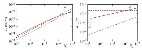
Fig. 9. Dependence of the luminosity (a) and the transverse beam size  $\sigma_x$  (b) on the number of ion beam particles: the cooled coasting ion beam below and above the phase transition (solid curves), the bunched ion beam with a constant emittance equal to the electron beam emittance (50 nm) (dashed curves), and the bunched ion beam with an emittance limited by the space charge (Laslett parameter) (dotted curves)
