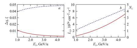
Fig. 6. Dependence of the parameters of the ion–ion collider with the coasting  $^{197}\mathrm{Au}^{79+}$  beams on the ion energy  $E_i$ ; beam emittances are  $11\,\pi\cdot\mathrm{mm}\cdot\mathrm{mrad}$ . a) Laslett parameter  $\Delta q$  (solid curve) and the BB parameter  $\xi$  (dashed curve); b) collider luminosity  $L_{ii}$  (solid curve) and the number of particles in a beam  $N_i$  (dashed curve)
