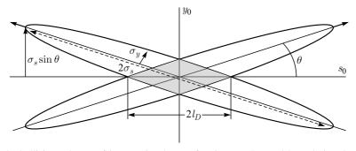
Fig. 3. Collision scheme of intersecting beams for  $\phi \gg 1$ ; the oval boundaries show the "1 sigma sizes"; colored grey is the particle interaction region
