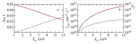
Fig. 5. Dependence of the parameters of the proton–proton collider on the proton energy  $E_p$ ;  $\Delta Q=0.05$ : a) Laslett parameter  $\Delta q$  (solid curve) and the BB parameter  $\xi$  (dashed curve); b) collider luminosity  $L_{pp}$  (solid curve) and the number of particles per bunch  $N_p$  (dashed curve)
