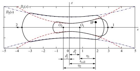
Fig. 1. Collision scheme of two bunches in the y=0 plane.  $O_{1,2}$  are the centers of the bunches;  $\eta_{1,2}$  are the distances of the interaction point (IP) of two particles from the centers of the bunches;  $s_{\text{coll}}$  is the same, from the origin;  $B_{1,2}(s)$  are the envelopes (beta functions) of the first and second beams
