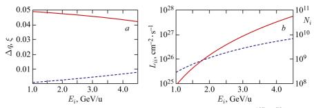
Fig. 4. Dependence of the parameters of the ion collider with the bunched  $^{197}\mathrm{Au}^{79+}$  beams on the ion energy  $E_i$ ;  $\Delta Q=0.05$ : a) Laslett parameter  $\Delta q$  (solid curve) and the BB parameter  $\xi$  (dashed curve); b) collider luminosity  $L_{ii}$  (solid curve) and the number of particles per bunch  $N_i$  (dashed curve)
