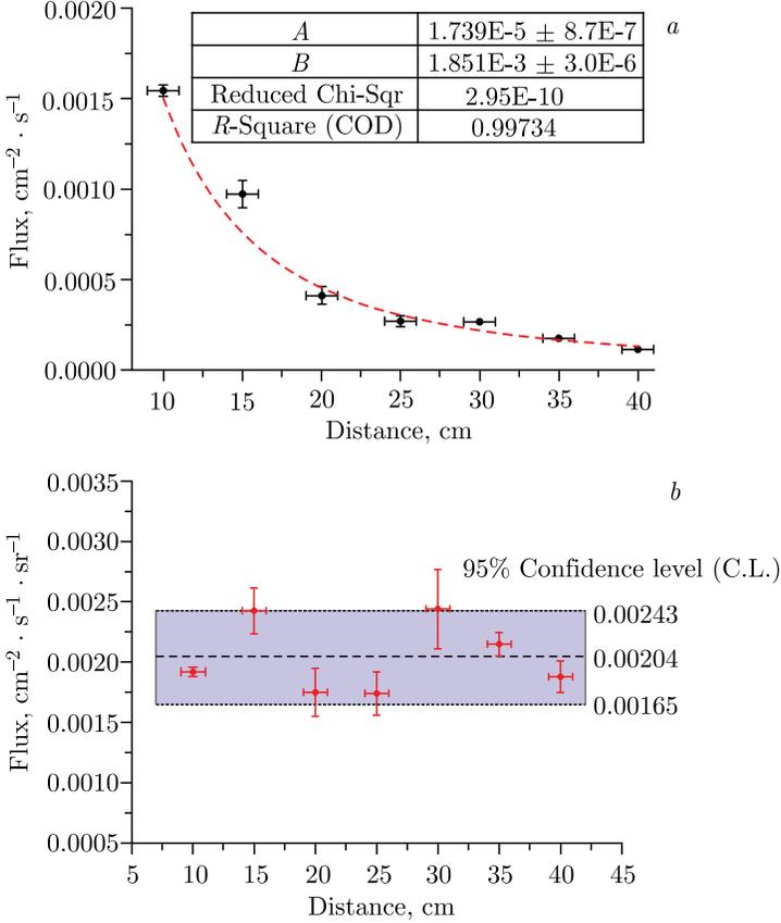
Fig. 3. *a*) The measured flux in coincidence mode for the different distance between detectors; *b*) the measured flux of muons normalized per steradian with an average value and C.L. at 95%
