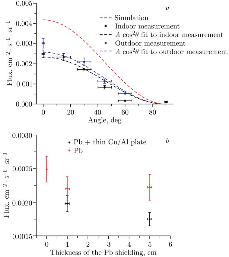
Fig. 4. *a*) The observed muon flux in coincidence indoors and outdoors. For the results, the  $A \cos^2\theta$  function is fitted with a dashed line. The red dashed line stands for the CORSIKA simulation; *b*) the muon flux for the different Pb shielding thickness and with/without thin Cu and Al plates between the master and slave detectors
