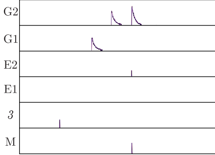
Fig. 6. Oscillogram of an experimental event with the release of two successive \gamma quanta. The scale of the figure in time is 20 \mu s
