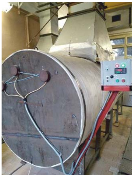
Fig. 8. Winding machine CH-10C-1200 Fig. 9. DLNP furnace for baking gallettes
