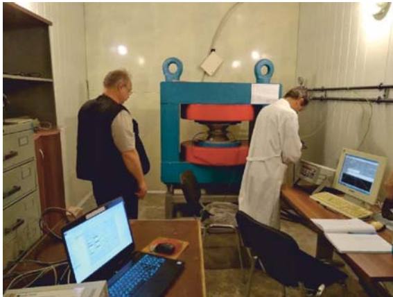
Fig. 10. Hall sensor calibration in the experiment dated 02.06.2021
